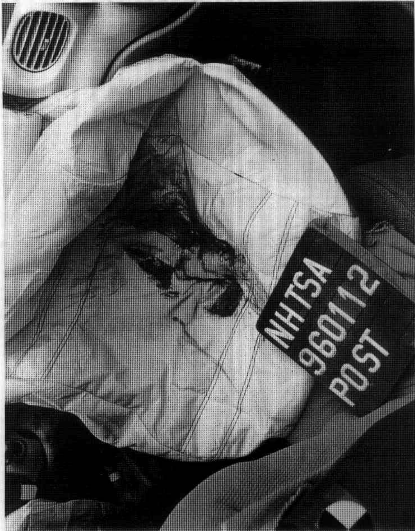
Figure A-28. Post-Test Passenger Dummy Head Contact - View 2
