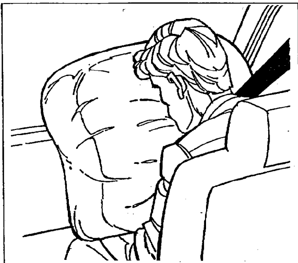
Inflated right front passenger side air bag
