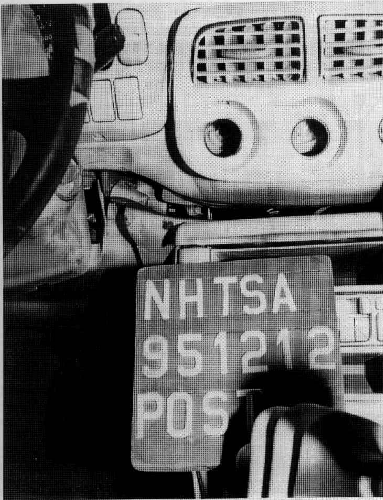
Figure A-25. Post-Test Driver Dummy Knee Contact - View 3
