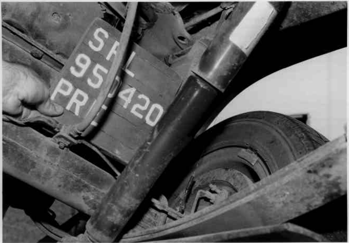
Figure A-9 Pre-Test Right Rear Suspension String Potentiometer View
