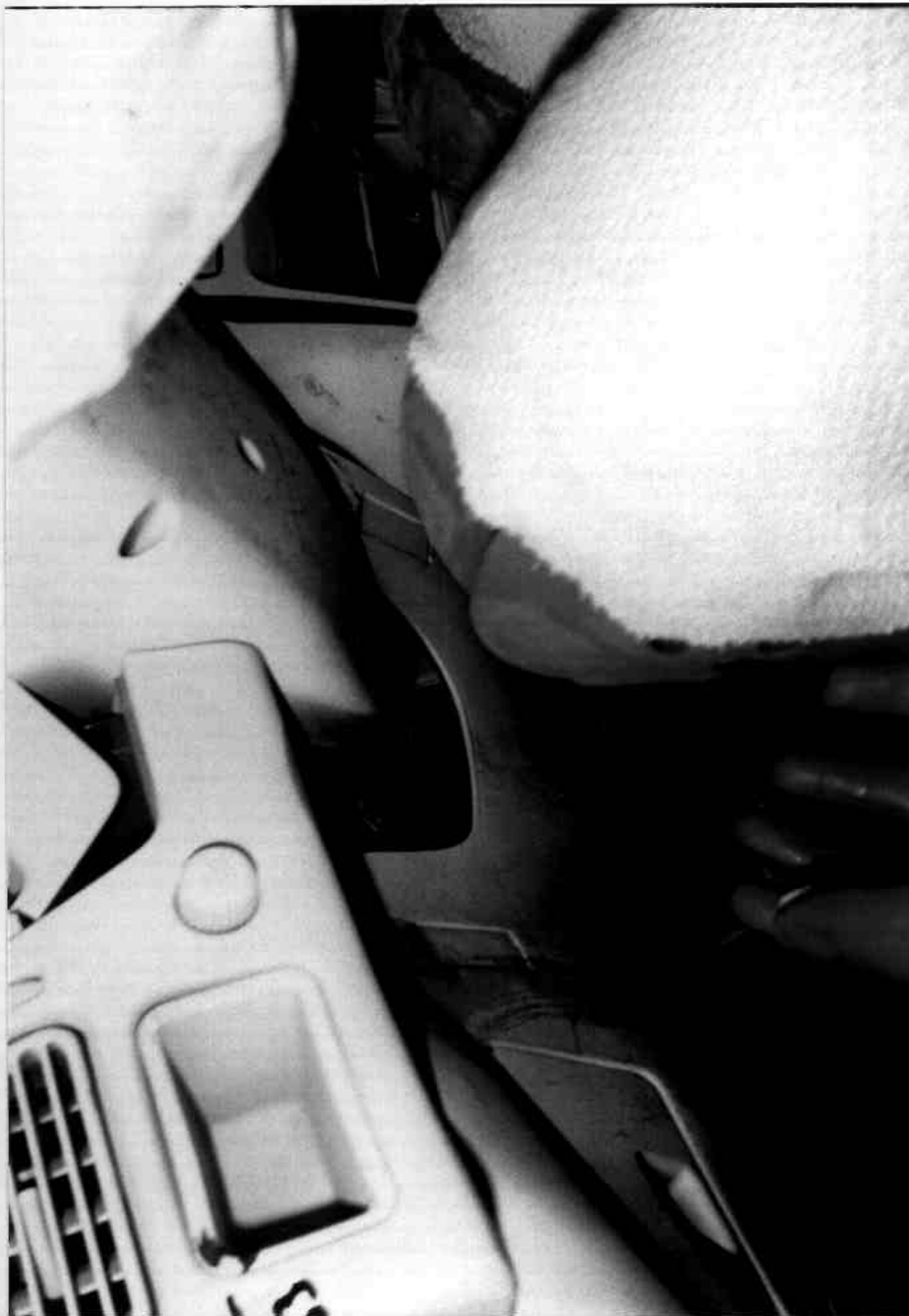
Figure A-17 POST-TEST DRIVER KNEE BOLSTER
