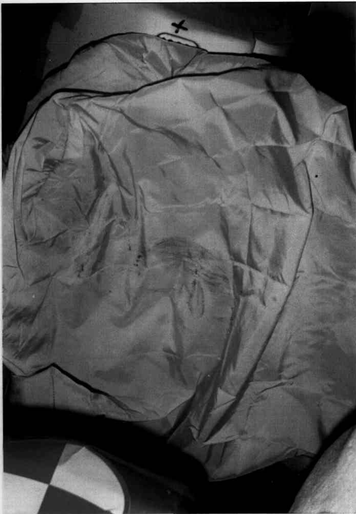
Figure A-23 POST-TEST PASSENGER AIRBAG VIEW
