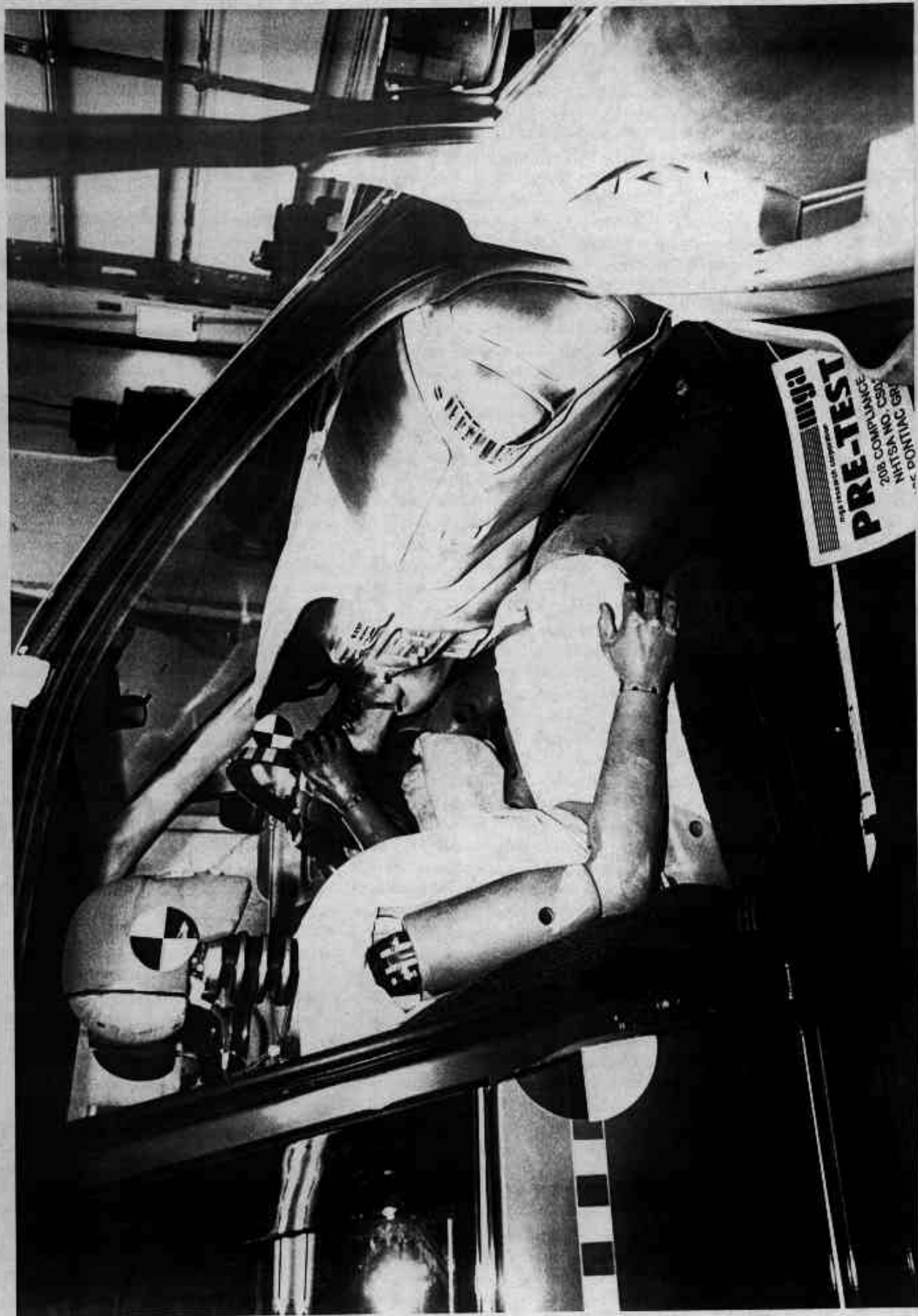
Photo No. A-37 - Pre-Test Passenger Dummy Position View (Door Open)
