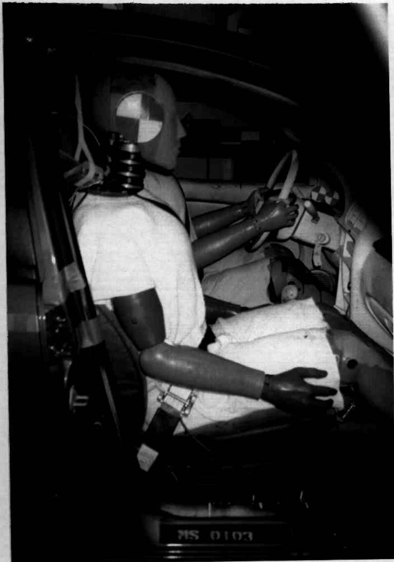
Figure A-31 PRE-TEST PASSENGER HEAD LOCATION A-33
