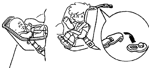
Installing a child restraint system to the rear center seat (Lap belt)
