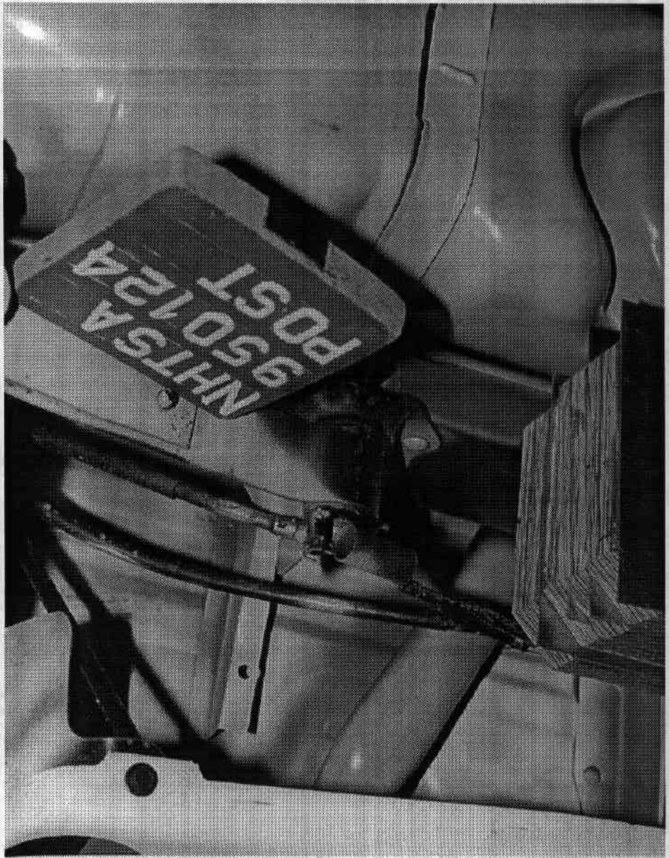
Figure A-20. Post-Test Fuel Filler Neck View
