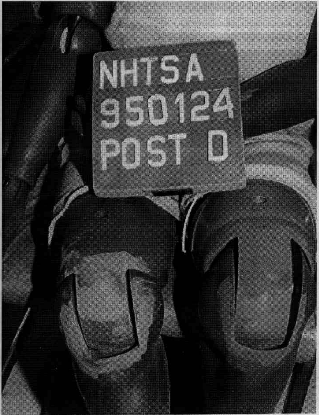
Figure A-41. Post-Test Driver Dummy Knee Contact - View I
