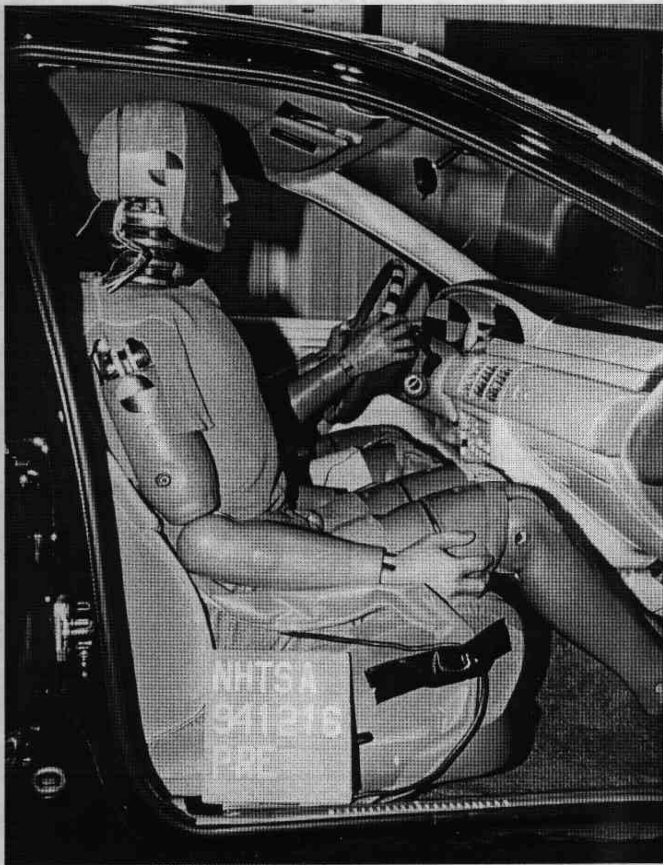
Figure A-15. Pre-Test Passenger Dummy & Vehicle Interior View
