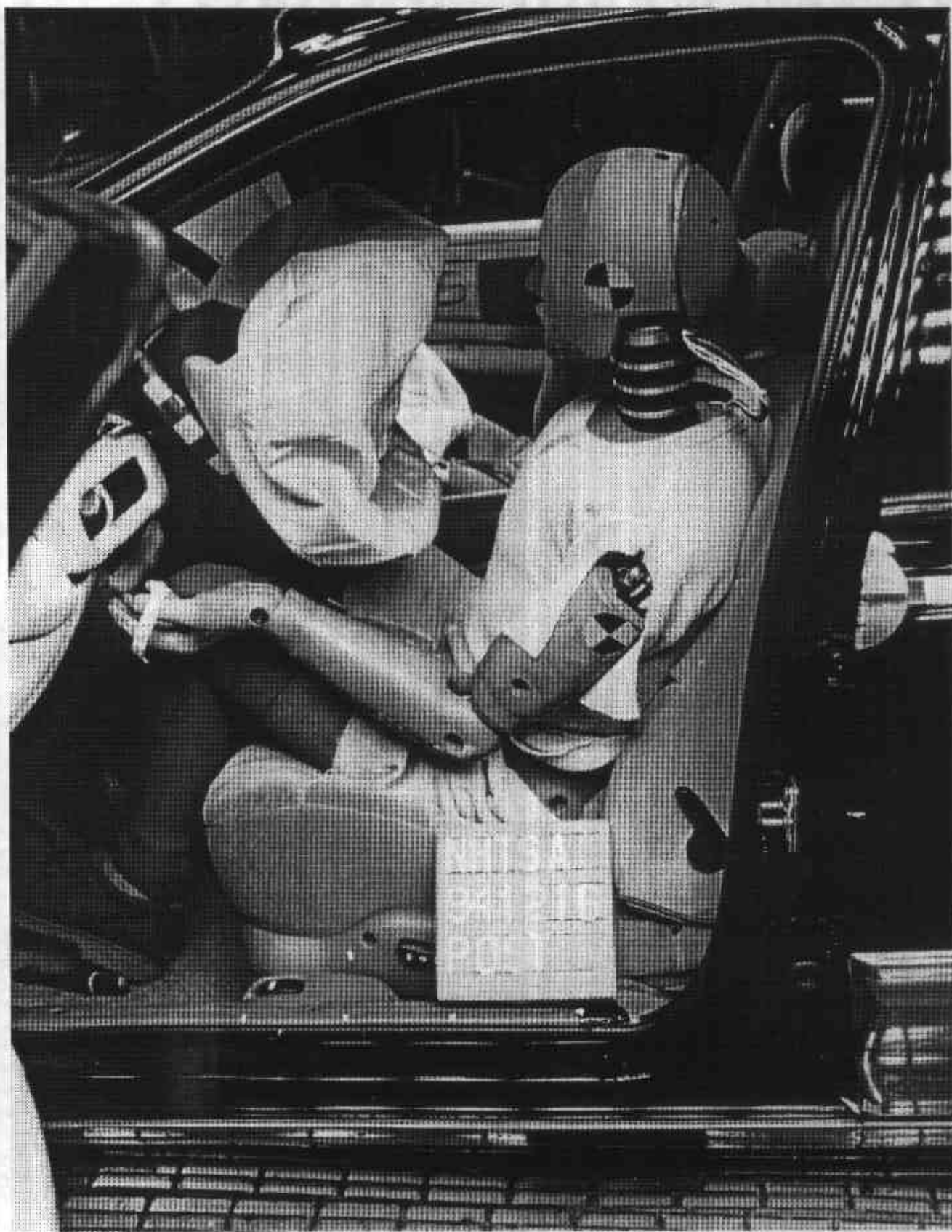
Figure A-14. Post-Test Driver Dummy & Vehicle Interior View A-15
