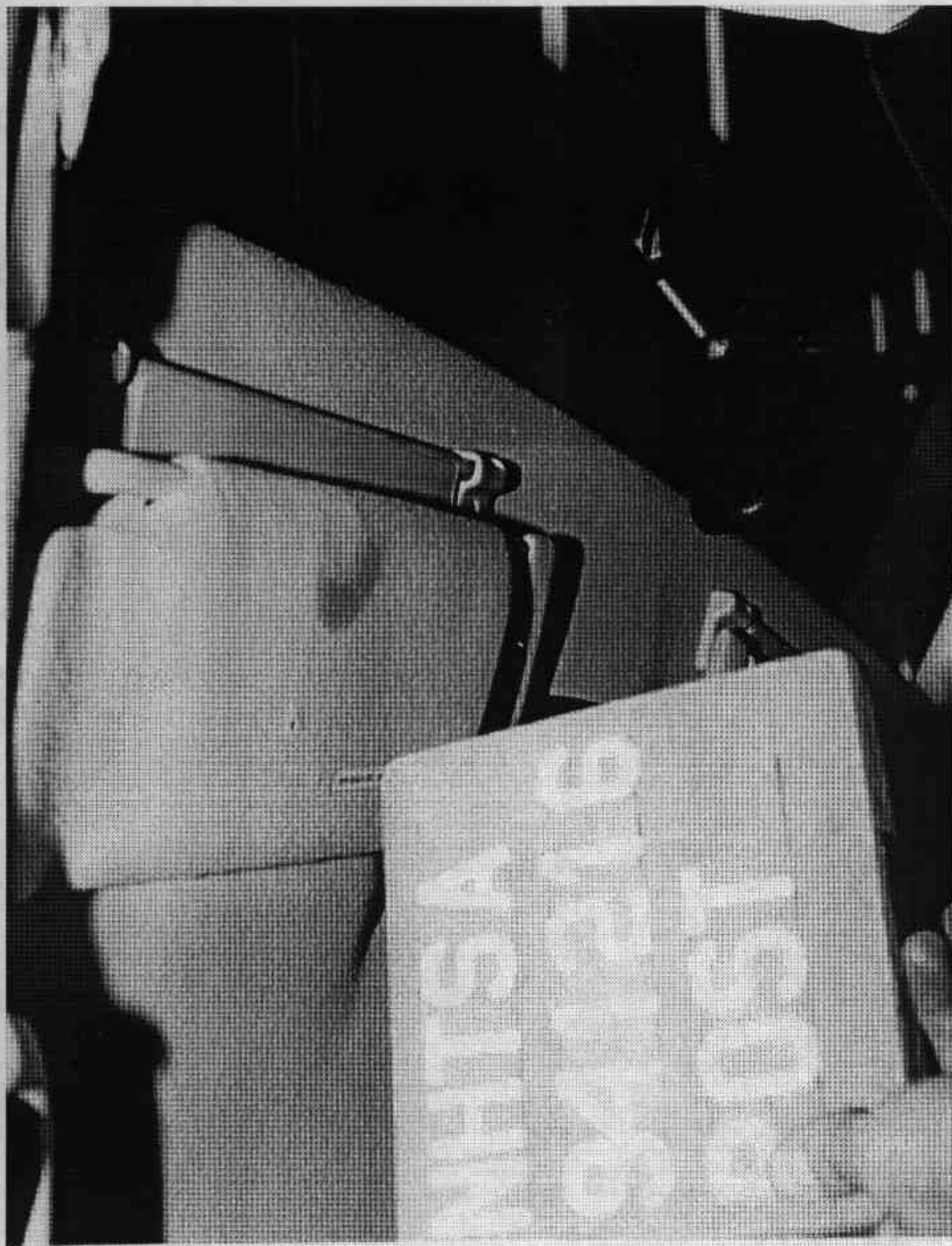
Figure A-25. Post-Test Passenger Dummy Head Contact - View 3
