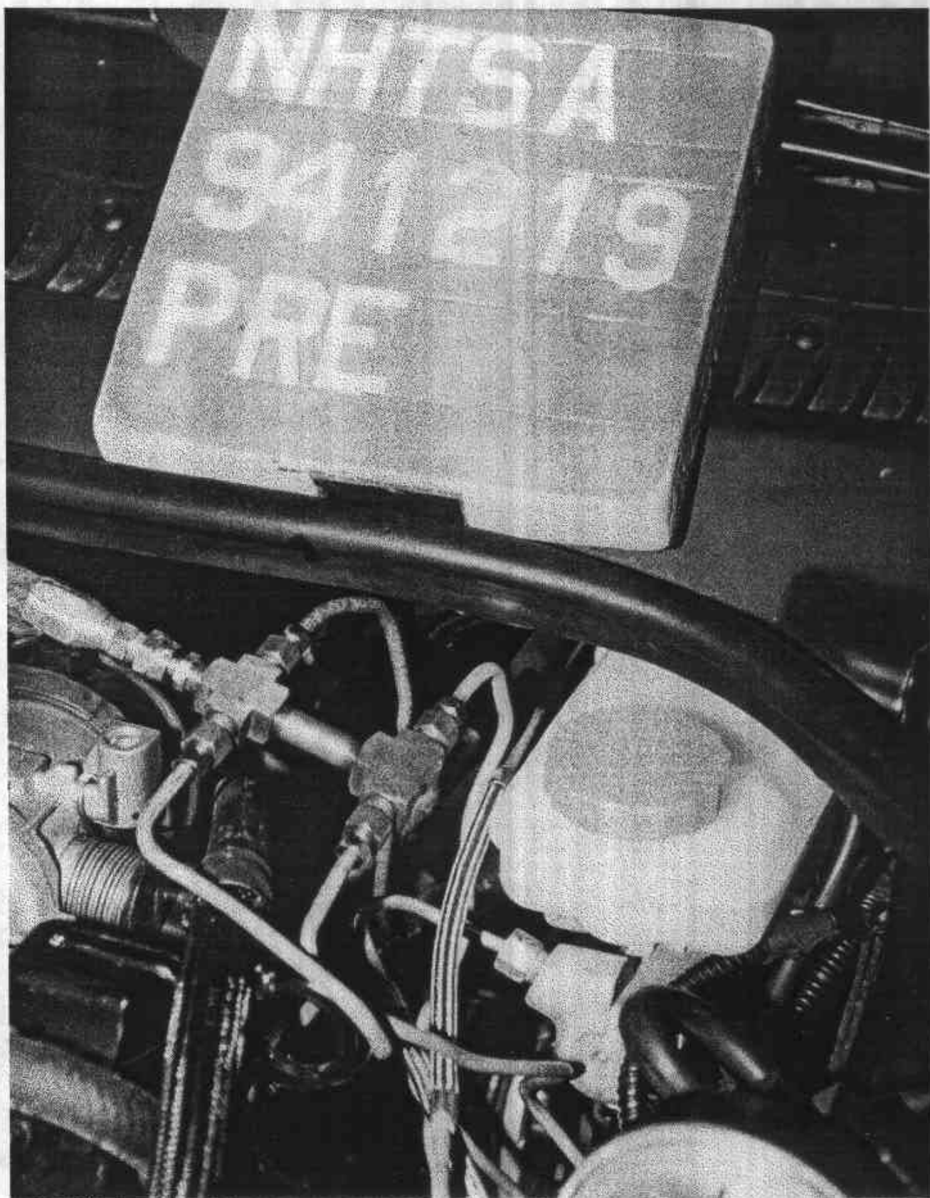
Figure A-12. Pre-Test Steering Column at Firewall View - Exterior
