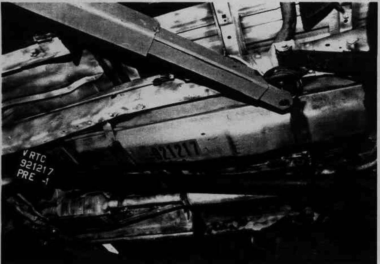
Figure A-16. PRE-TEST FUEL TANK VIEW
