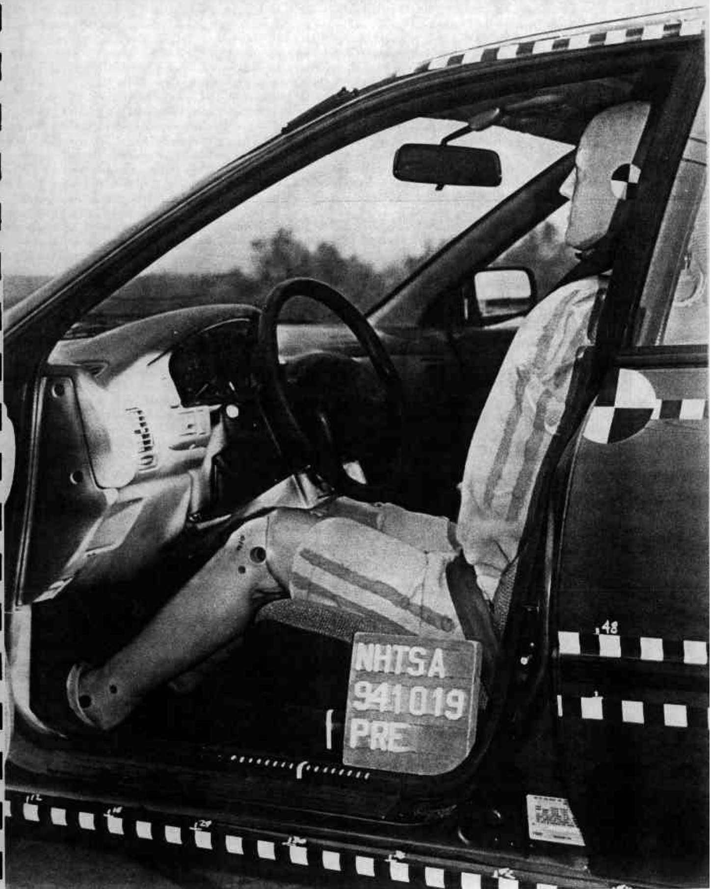
Figure A-25 Pre-test Driver Dummy & Vehicle Interior - View 1 A-26
