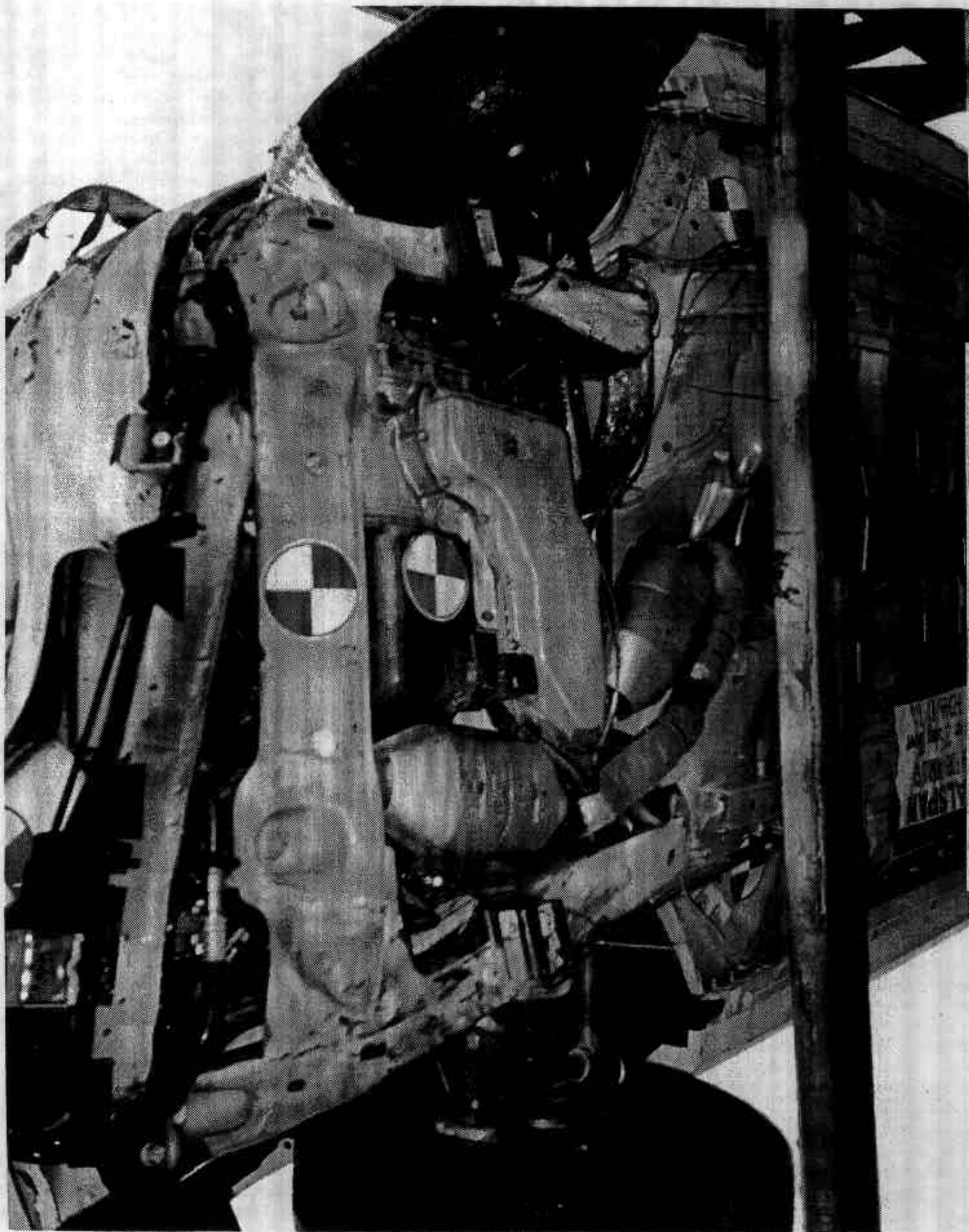
FIGURE A-27 POST-TEST UNDERBODY FRONT VIEW
