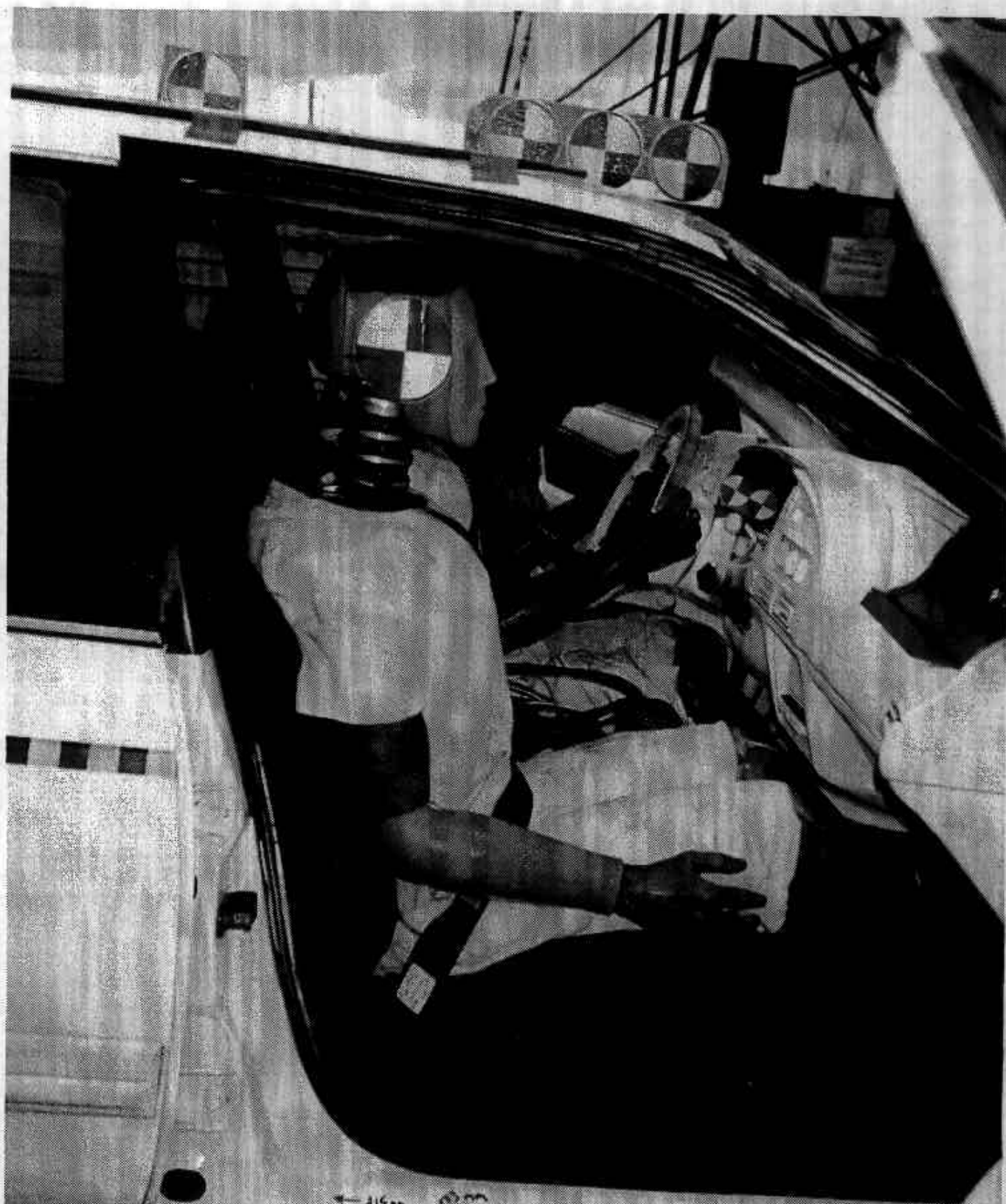
FIGURE A-39 PRE-TEST PASSENGER POSITION VIEW
