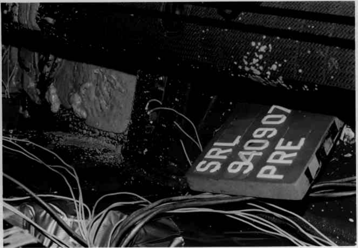
Figure A-11 PRE-TEST VEHICLE CENTER OF GRAVITY ACCELEROMETER VIEW
