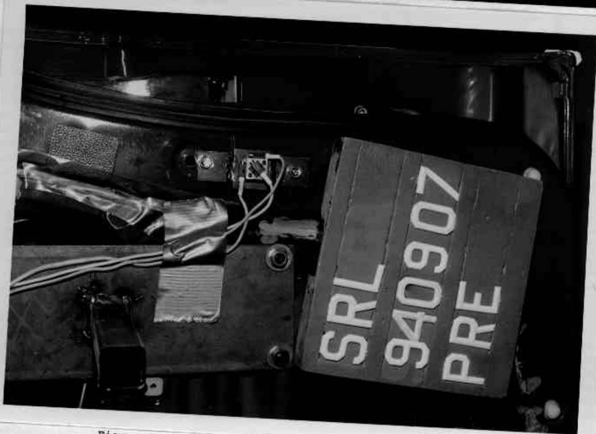
Figure A-13 PRE-TEST RIGHT DOOR ACCELEROMETER VIEW
