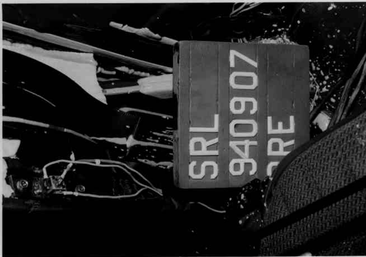
Figure A-15 PRE-TEST RIGHT B-PILLAR ACCELEROMETER VIEW
