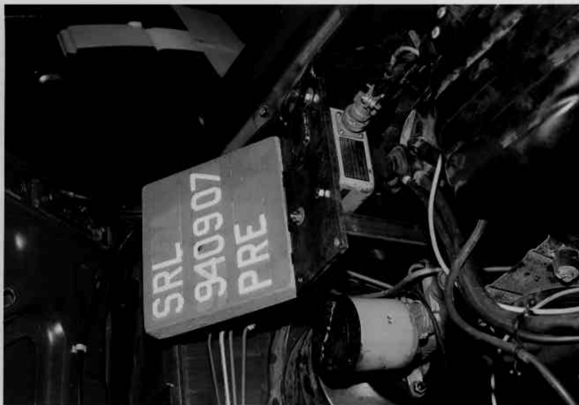
Figure A-6 PRE-TEST LEFT FRONT SUSPENSION STRING POTENTIOMETER VIEW
