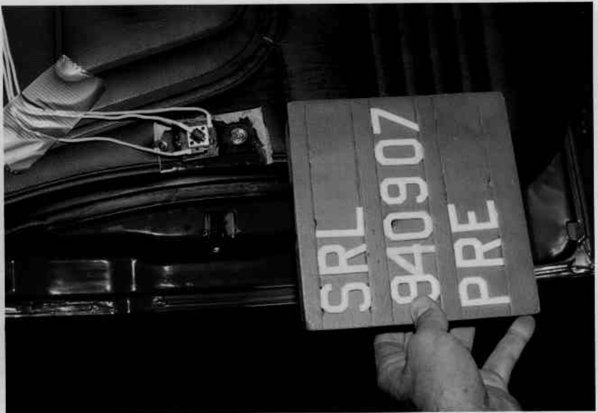
Figure A-12 PRE-TEST LEFT DOOR ACCELEROMETER VIEW
