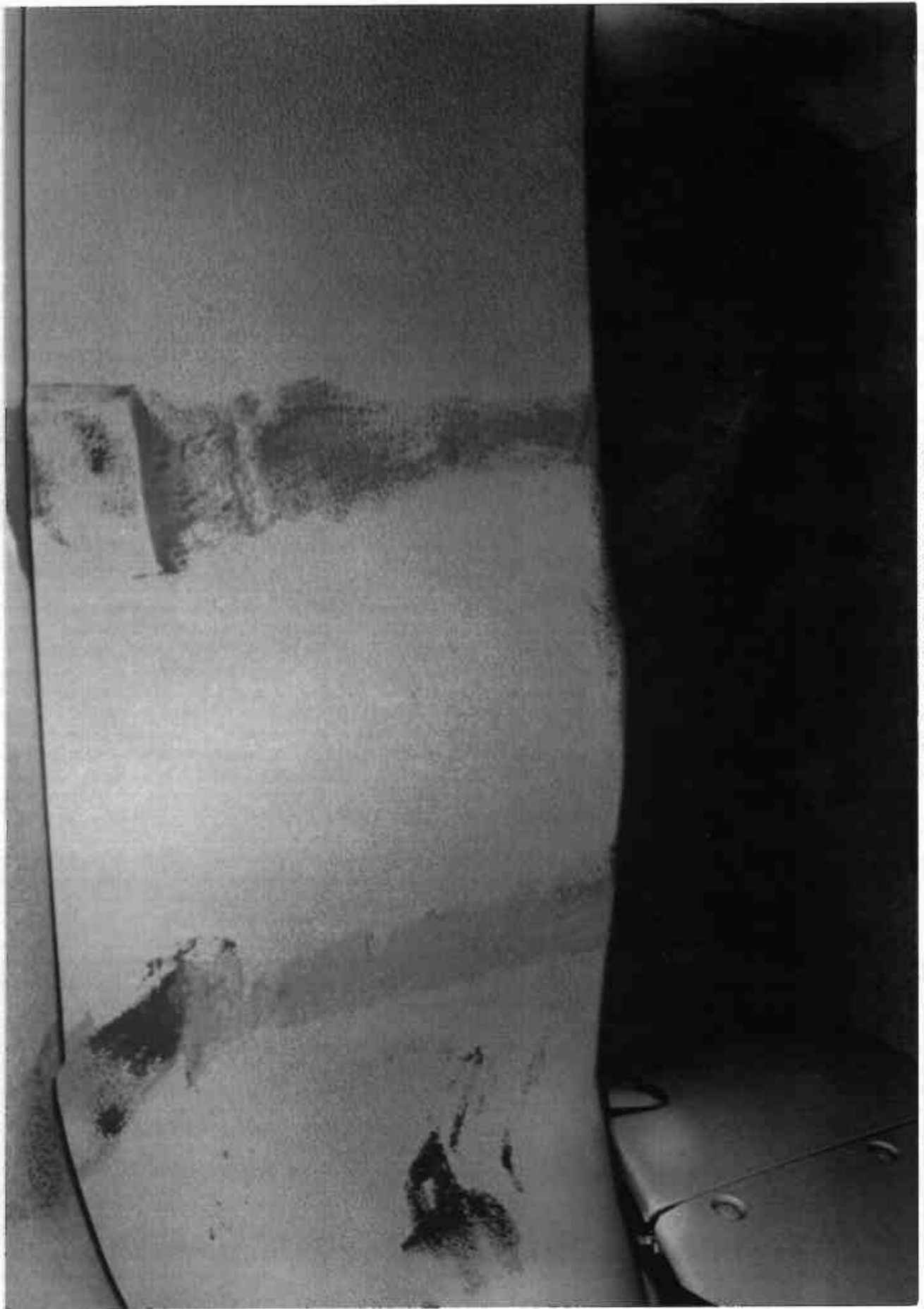
Figure A-38 POST-TEST PASSENGER KNEE BOLSTER
