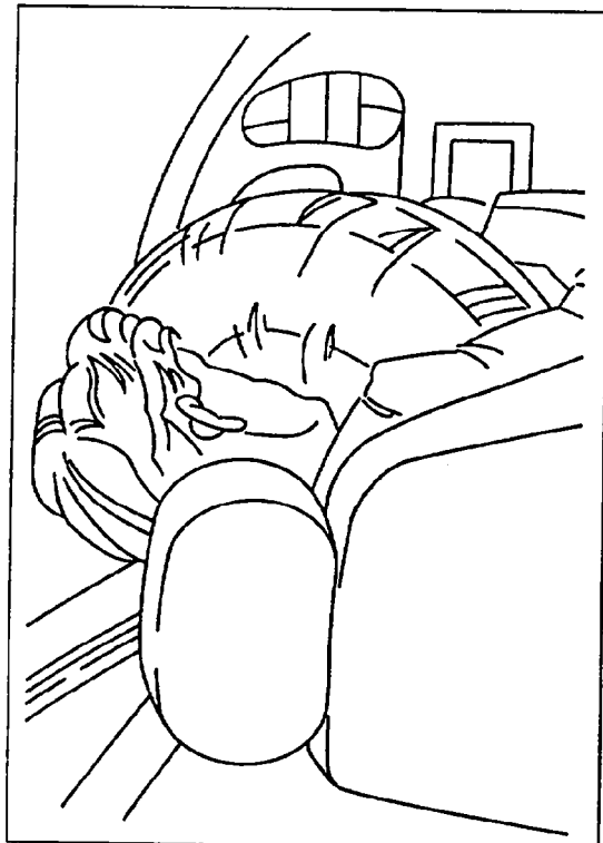
Inflated driver-side supplemental air bag
