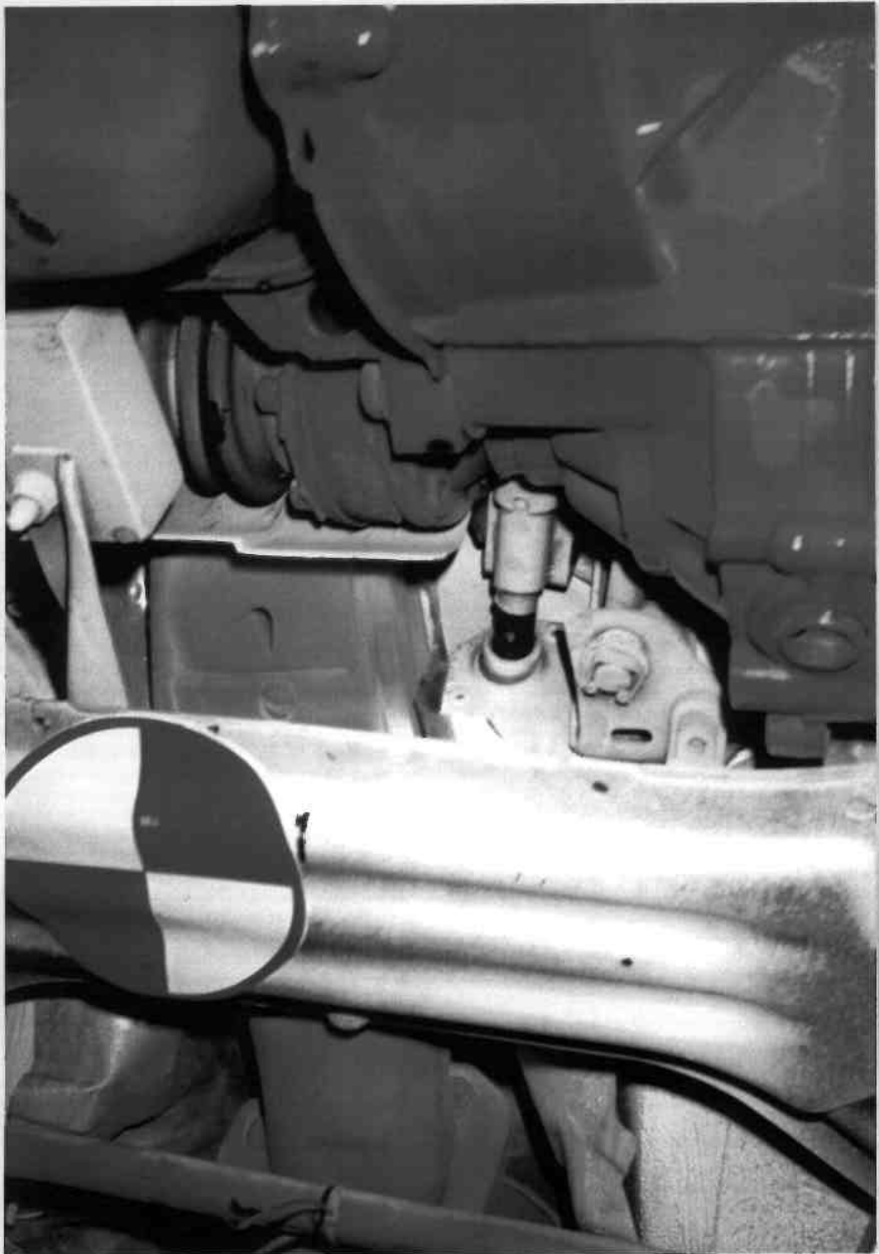
Figure A-14 POST-TEST UNDERBODY STEERING SHAFT VIEW
