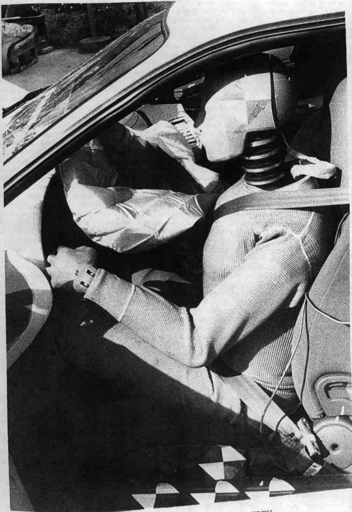
POSTTEST DRIVER ATD POSITION VIEW
