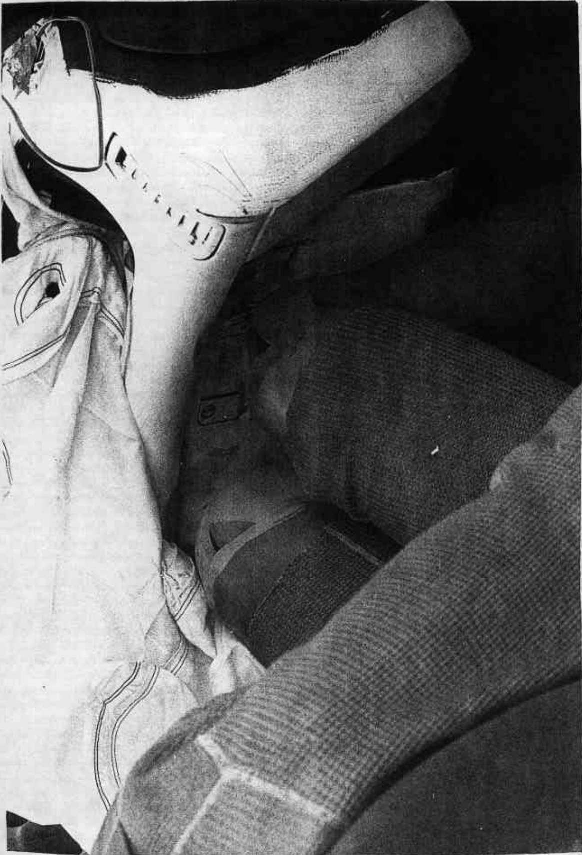
POSTEST PASSENGER ATD KNEE CONTACT AREA
