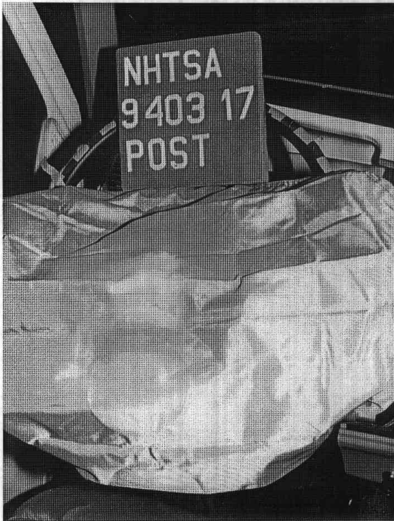
Figure A-50. Post-test Driver Dummy Head Contact - View 2 A-51
