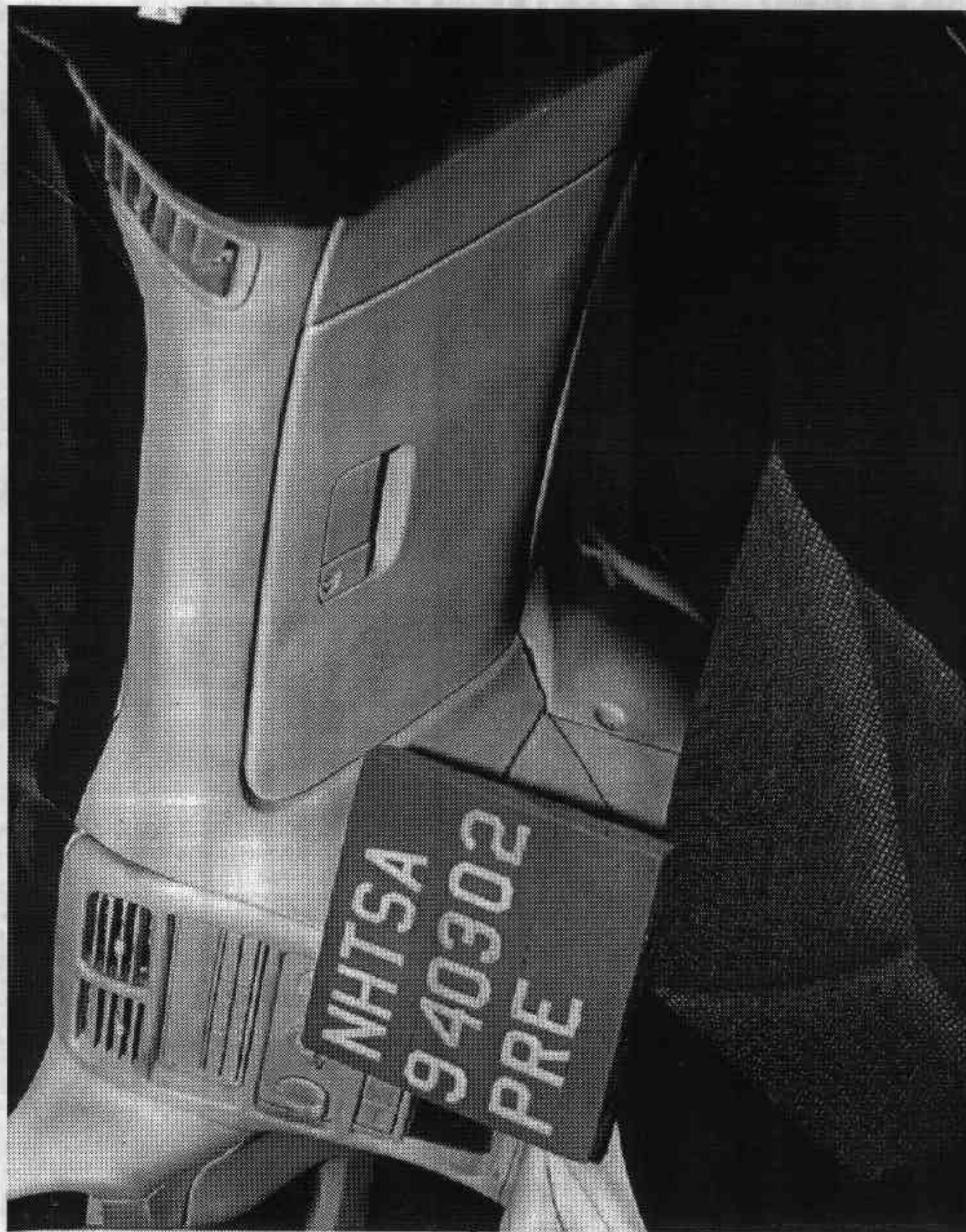
Figure A-28. Pre-test Passenger's Knee Bolster View A-29
