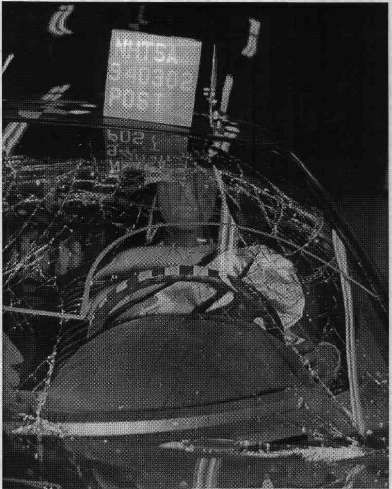
Figure A-34, Post-test Driver Dummy Position - View 1 A-35
