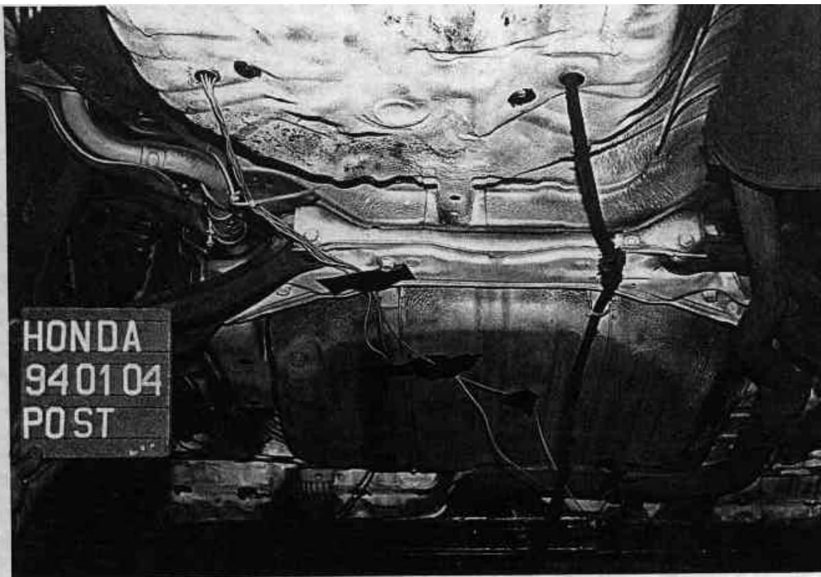
Figure A-27 POST-TEST FUEL FILLER NECK AND FUEL TANK VIEW
