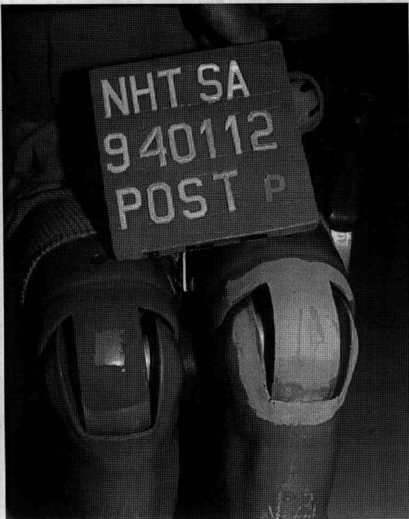
Fig. A-56. POST-TEST PASSENGER DUMMY KNEE CONTACT - VIEW 1 A-57 940112
