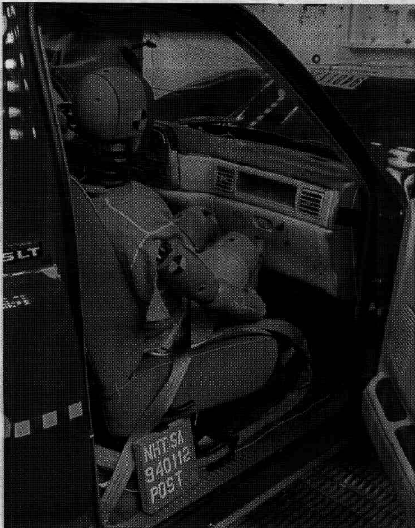
Fig. A-48. POST-TEST PASS. DUMMY & VEHICLE INTERIOR - VIEW 2
