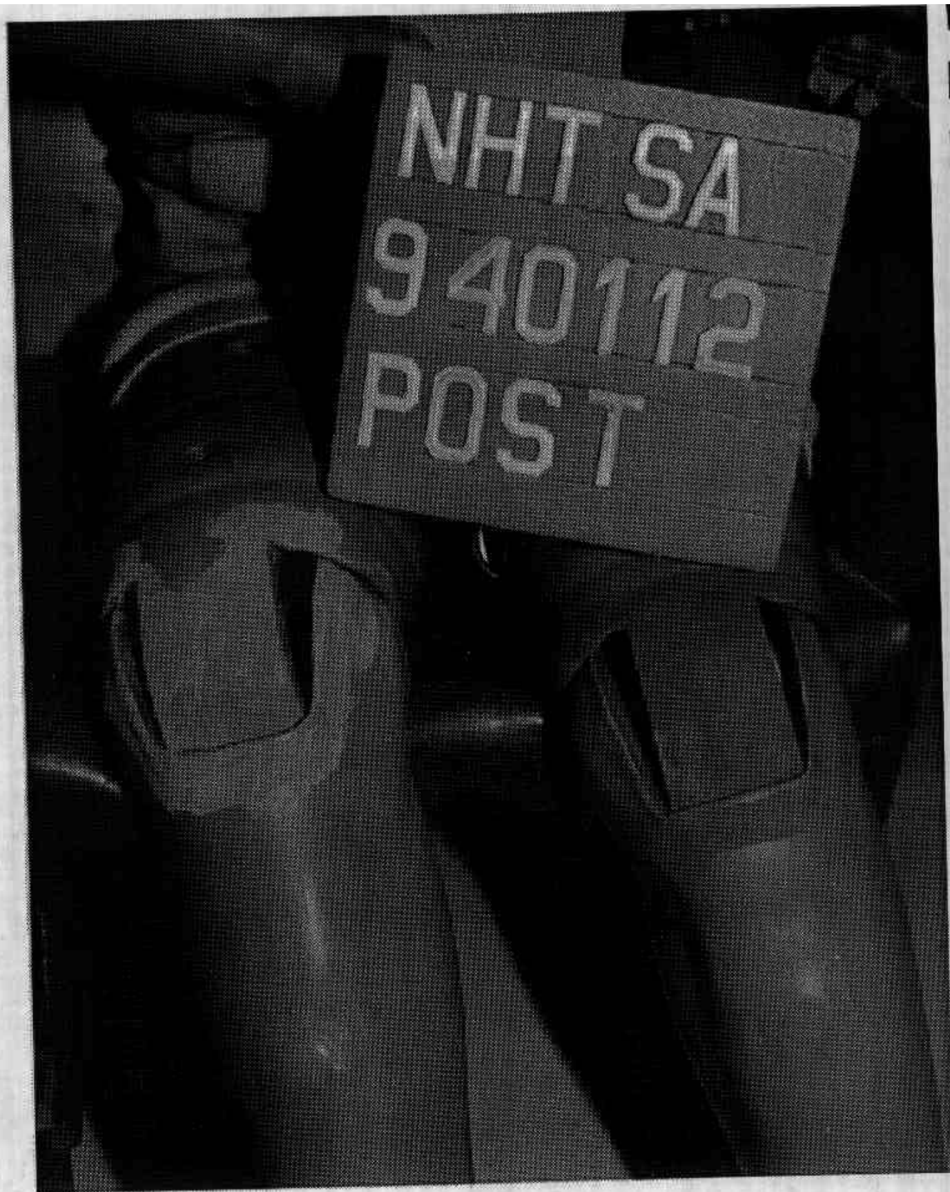
Figure A-52. POST-TEST DRIVER DUMMY KNEE CONTACT - VIEW 1
