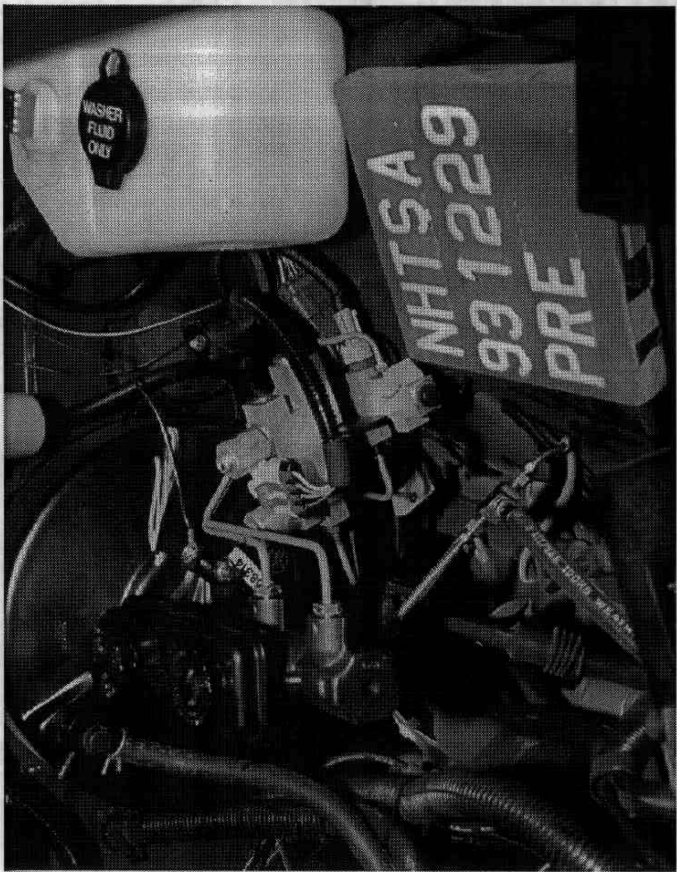
Figure A-56. PRE-TEST STEERING COLUMN SHAFT AT FIREWALL
