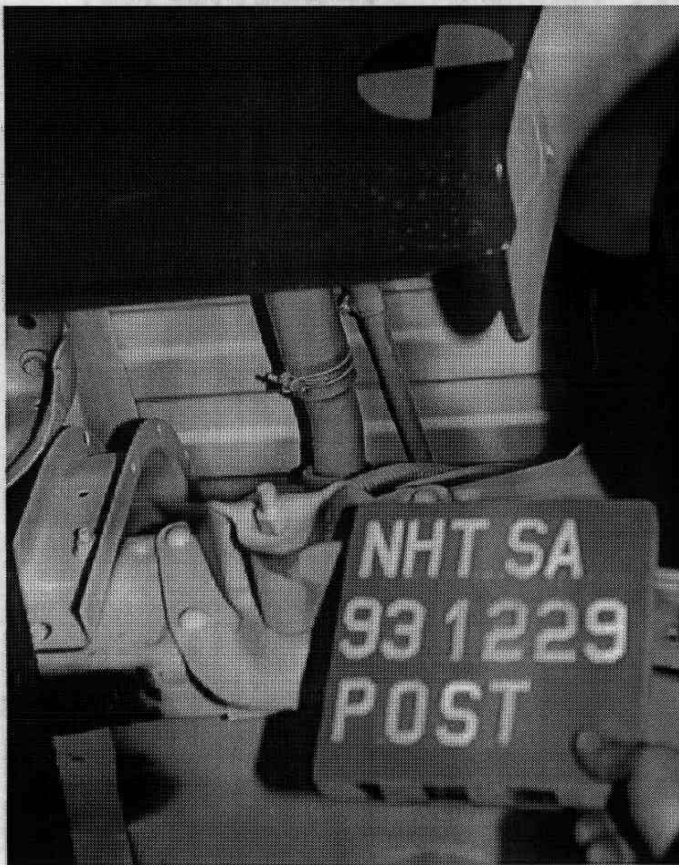
Figure A-20. POST-TEST FUEL FILLER NECK VIEW
