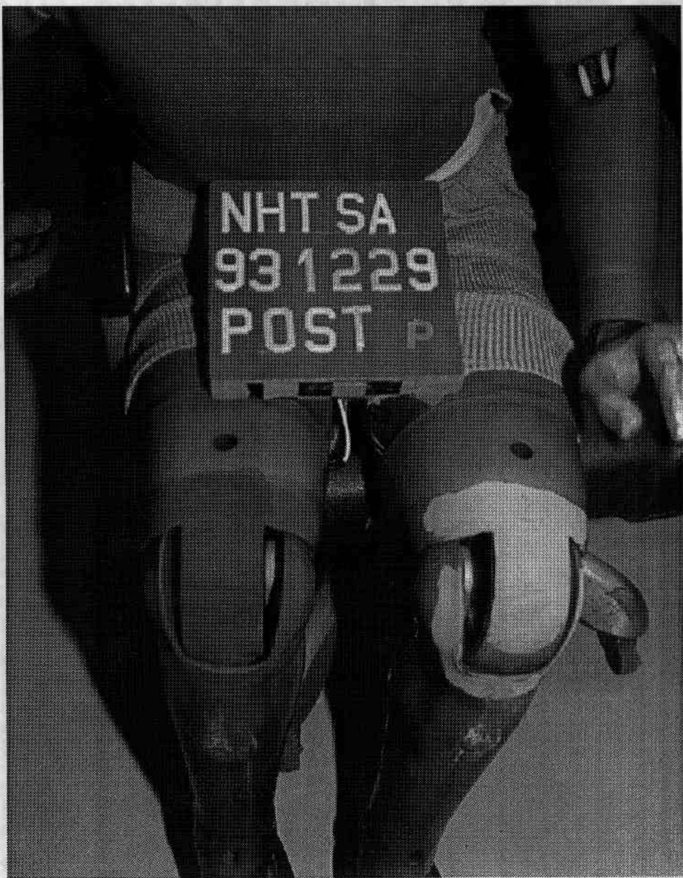
Fig. A-50. POST-TEST PASSENGER DUMMY KNEE CONTACT - VIEW 1 A-51 931229
