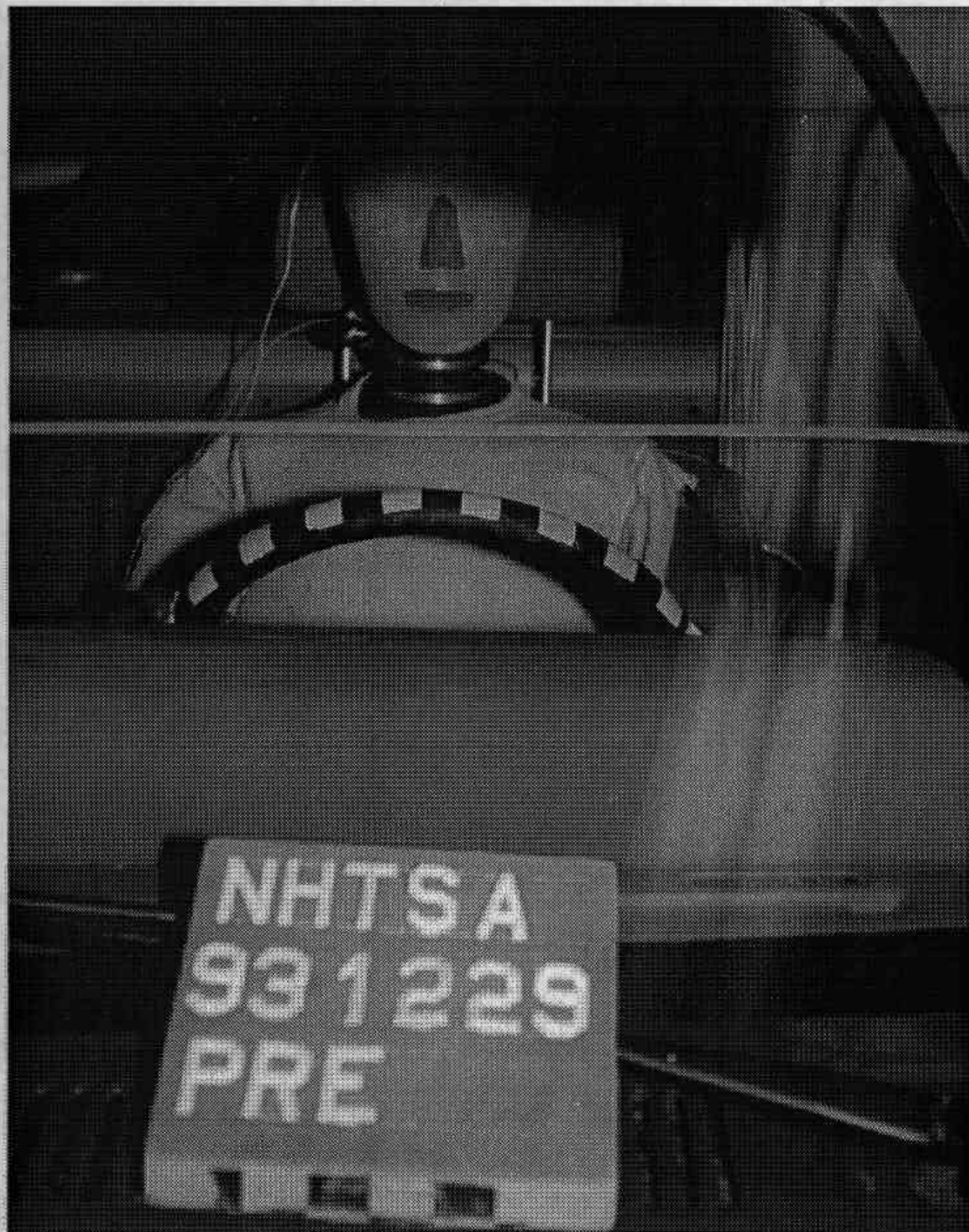
Figure A-29. PRE-TEST DRIVER DUMMY POSITION - VIEW 1
