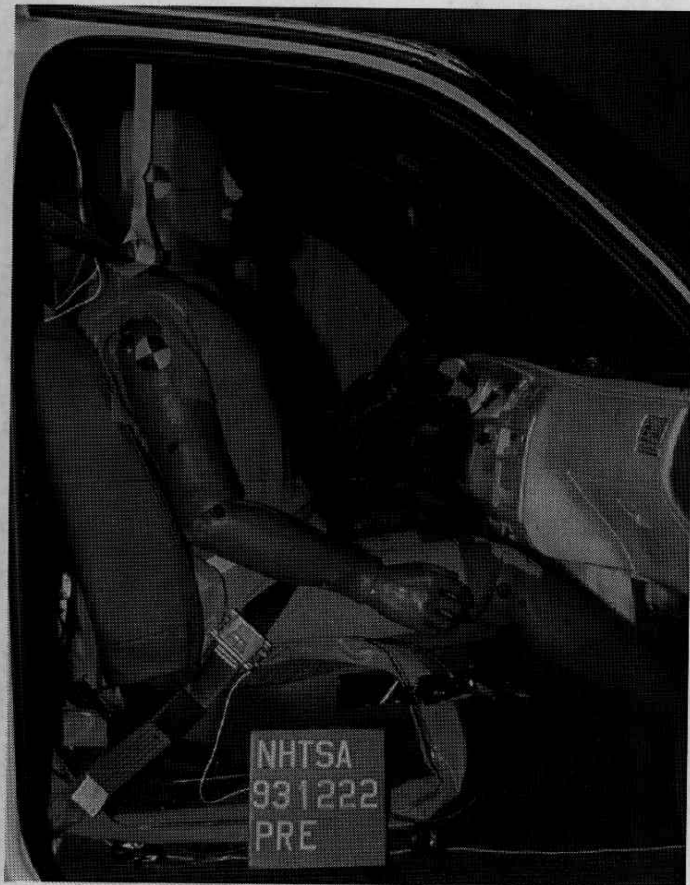
Fig. A-35. PRE-TEST PASS.DUMMY & VEHICLE INTERIOR - VIEW 1
