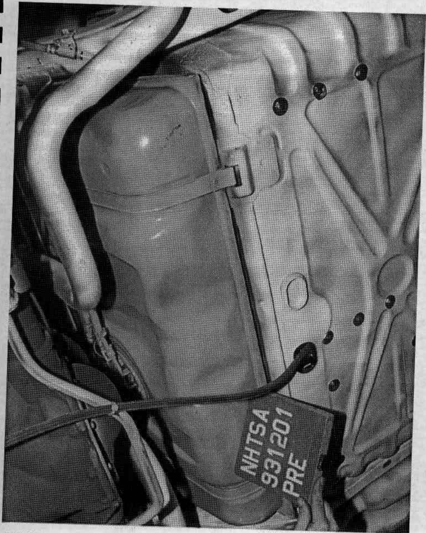
Figure A-21. PRE-TEST FUEL TANK VIEW A-22
