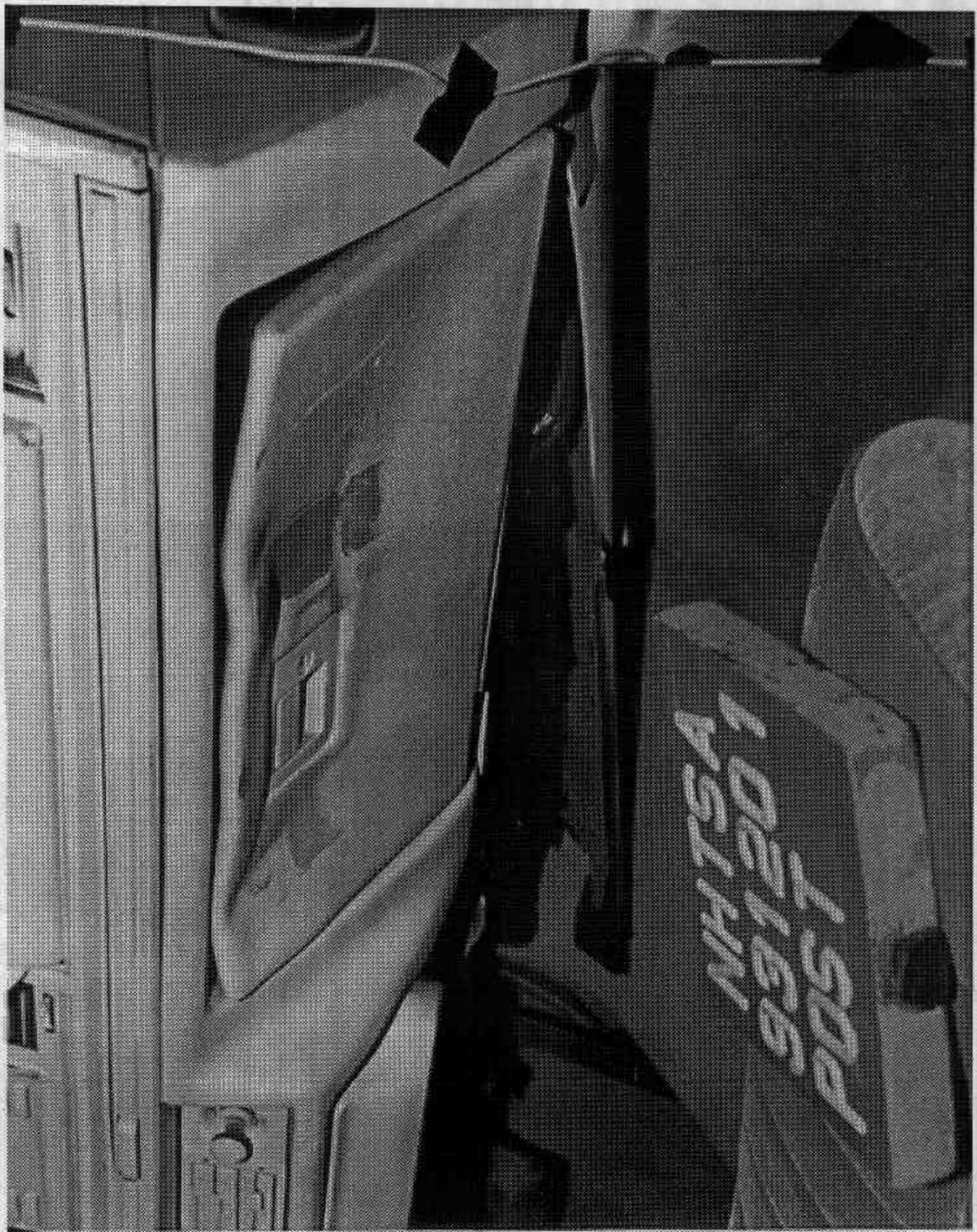
Figure A-52. POST-TEST PASSENGER DUMMY KNEE CONTACT - VIEW 2
