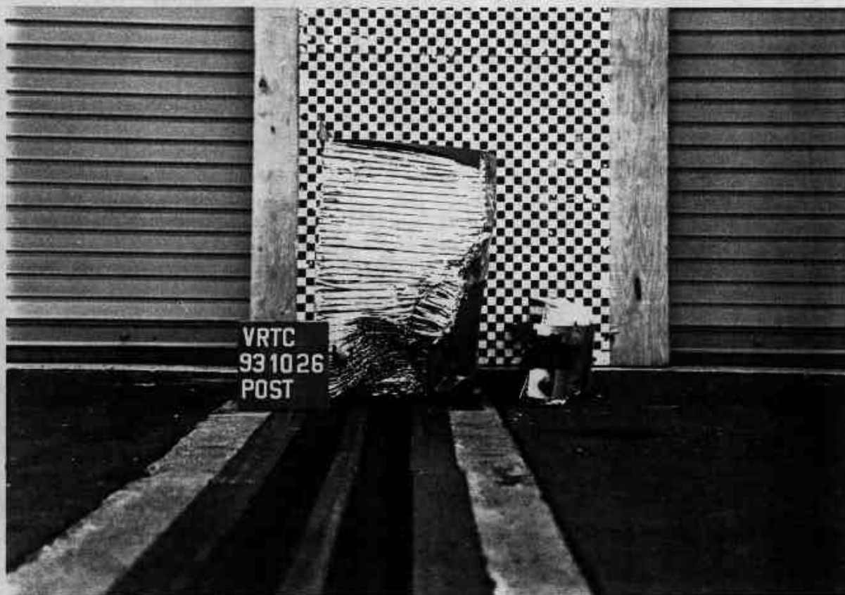
Figure A-31 POST-TEST VEHICLE IMPACTOR FACE - RIGHT SIDE VIEW
