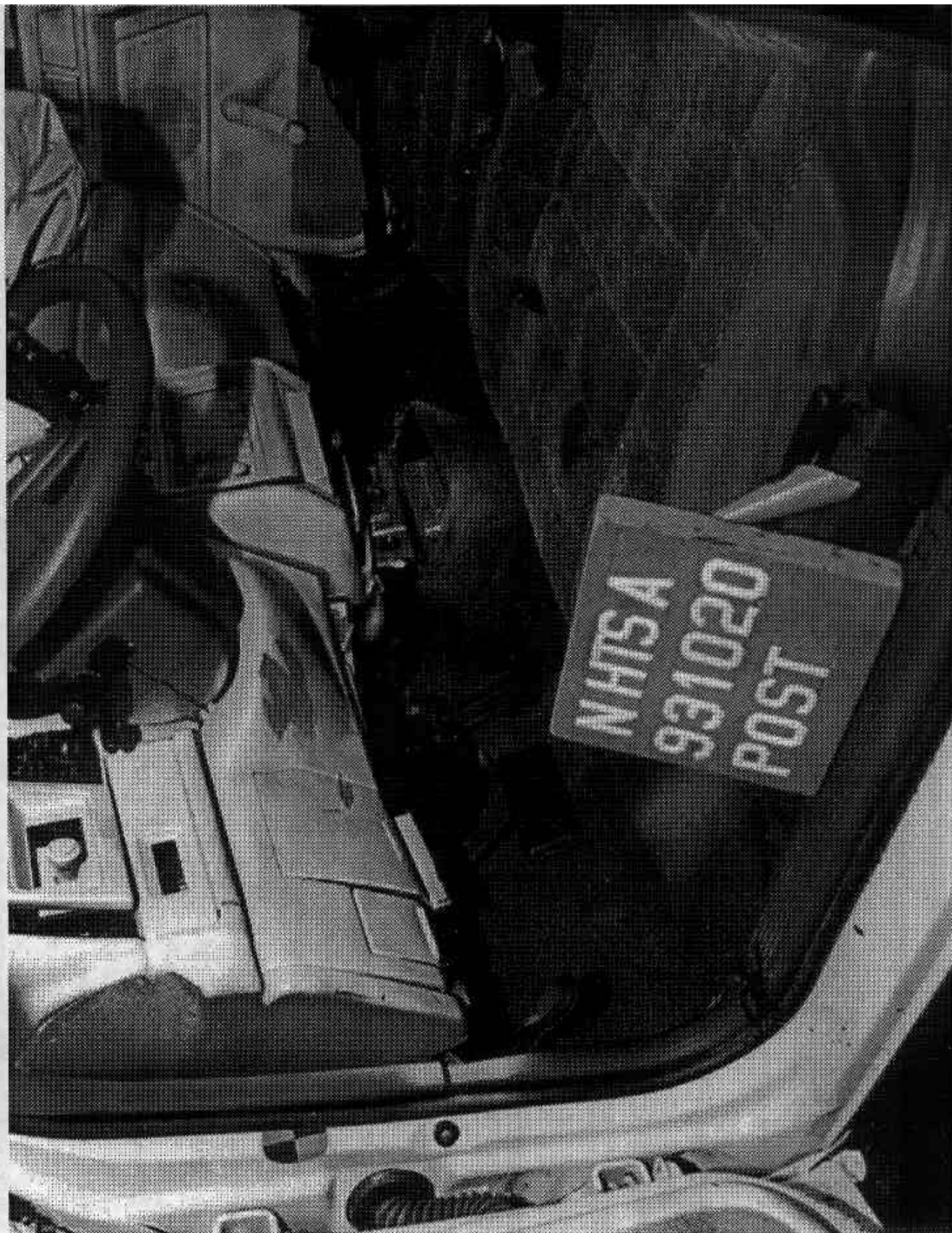
Figure A-40. POST-TEST DRIVER DUMMY KNEE CONTACT - VIEW 2 A-41 931020
