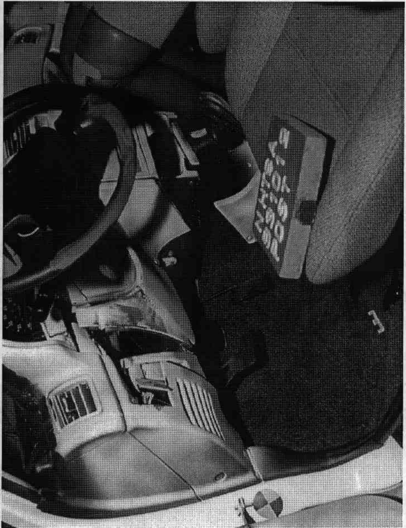
Figure A-43. POST-TEST DRIVER DUMMY CHEST AND KNEE CONTACT VIEW
