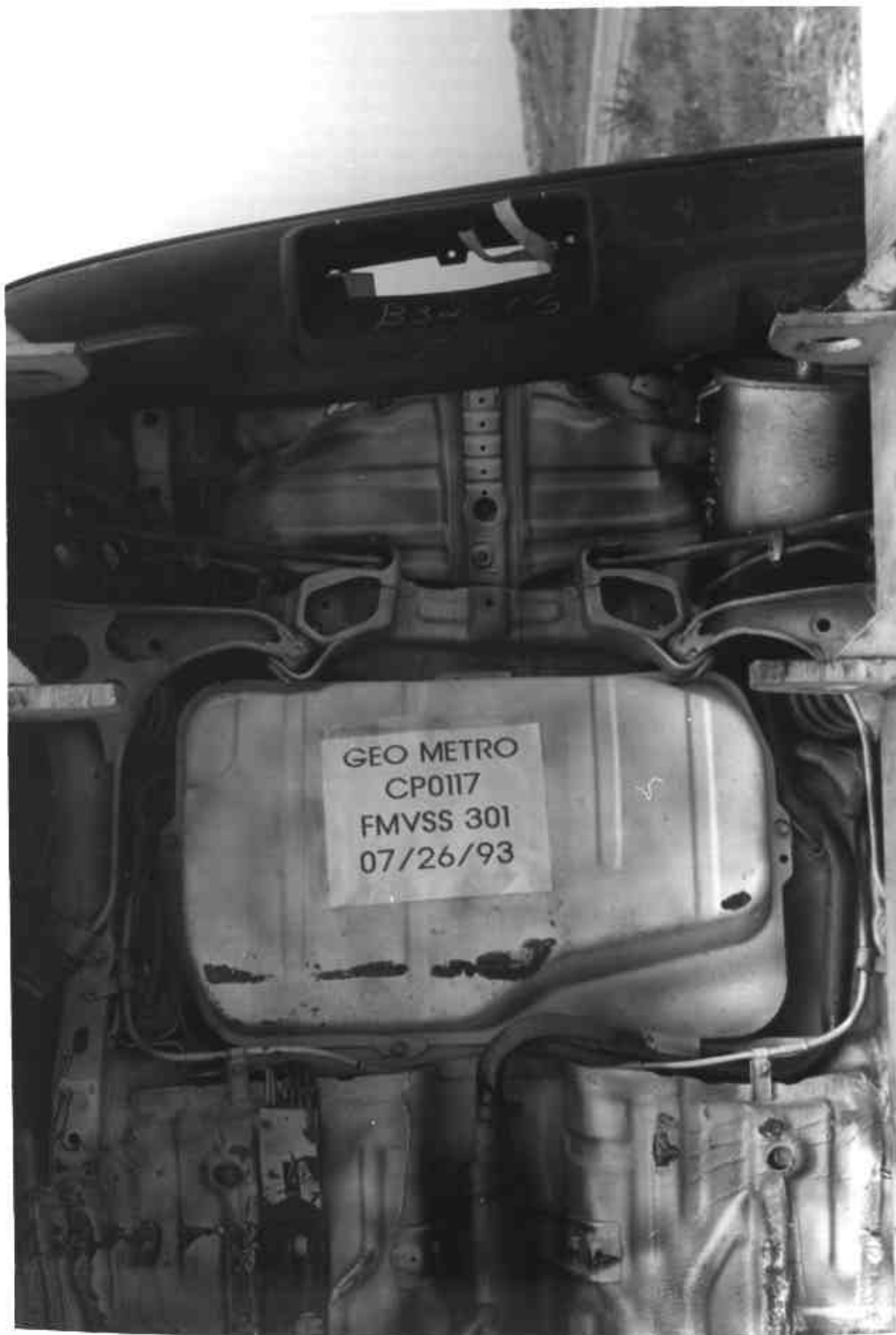
FIGURE 5-12 POSTTEST FUEL TANK CLOSEUP VIEW
