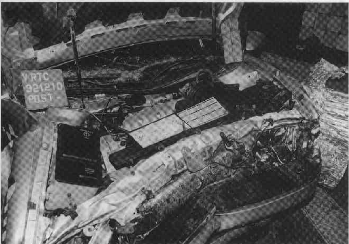
Figure A-14. POST-TEST ENGINE COMPARTMENT VIEW
