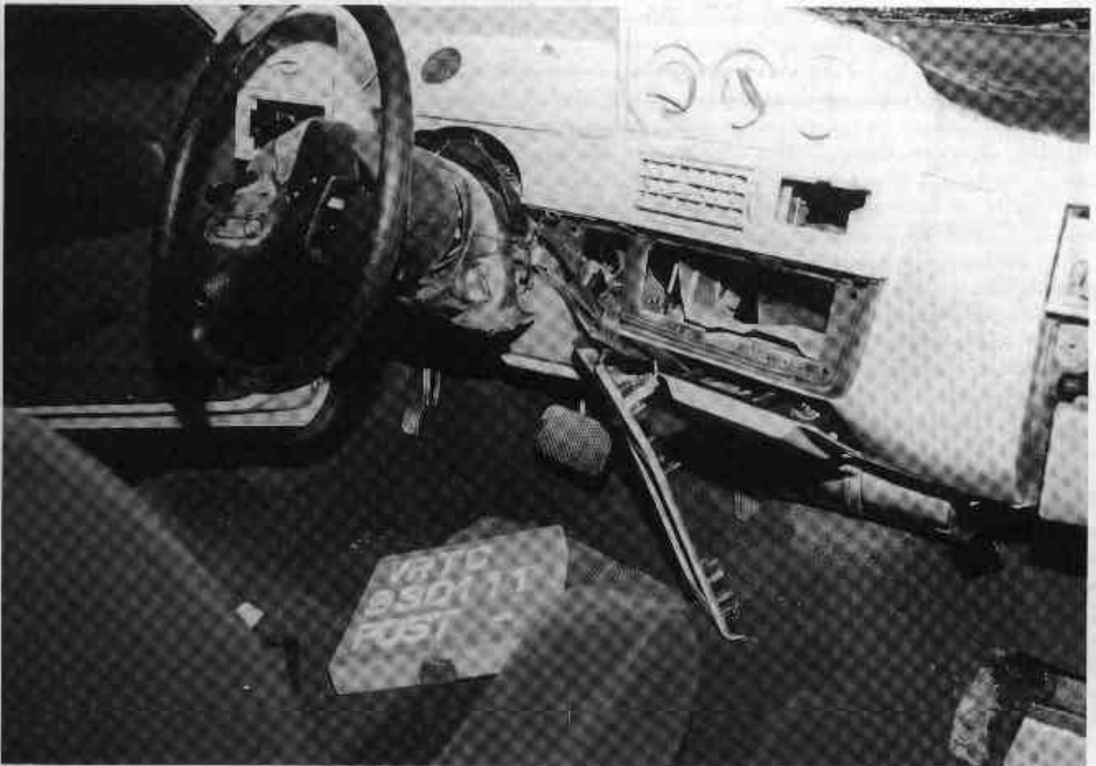
Figure A-22. POST-TEST DUMMY HEAD & KNEE CONTACT - VIEW 1
