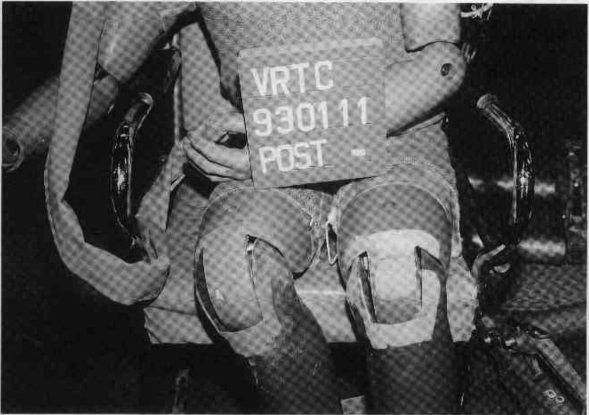
Figure A-21. POST-TEST DUMMY KNEE CONTACT VIEW
