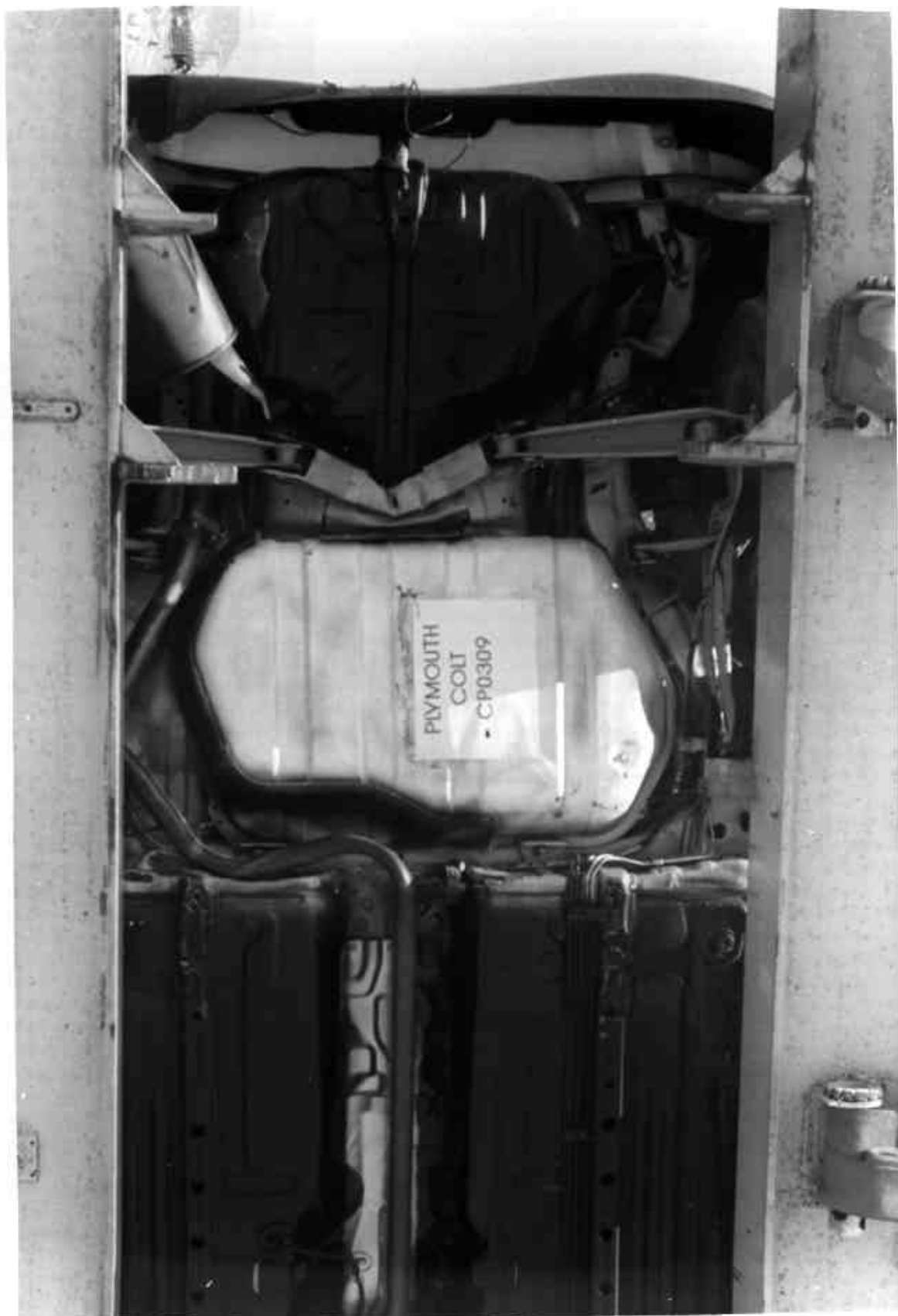
FIGURE 5-12 POSTTEST FUEL TANK CLOSEUP VIEW
