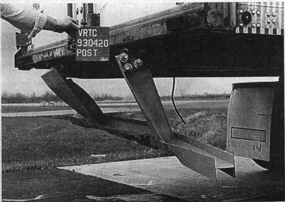
Figure A-40. POST-TEST UNDERRIDE GUARD - VIEW 3
