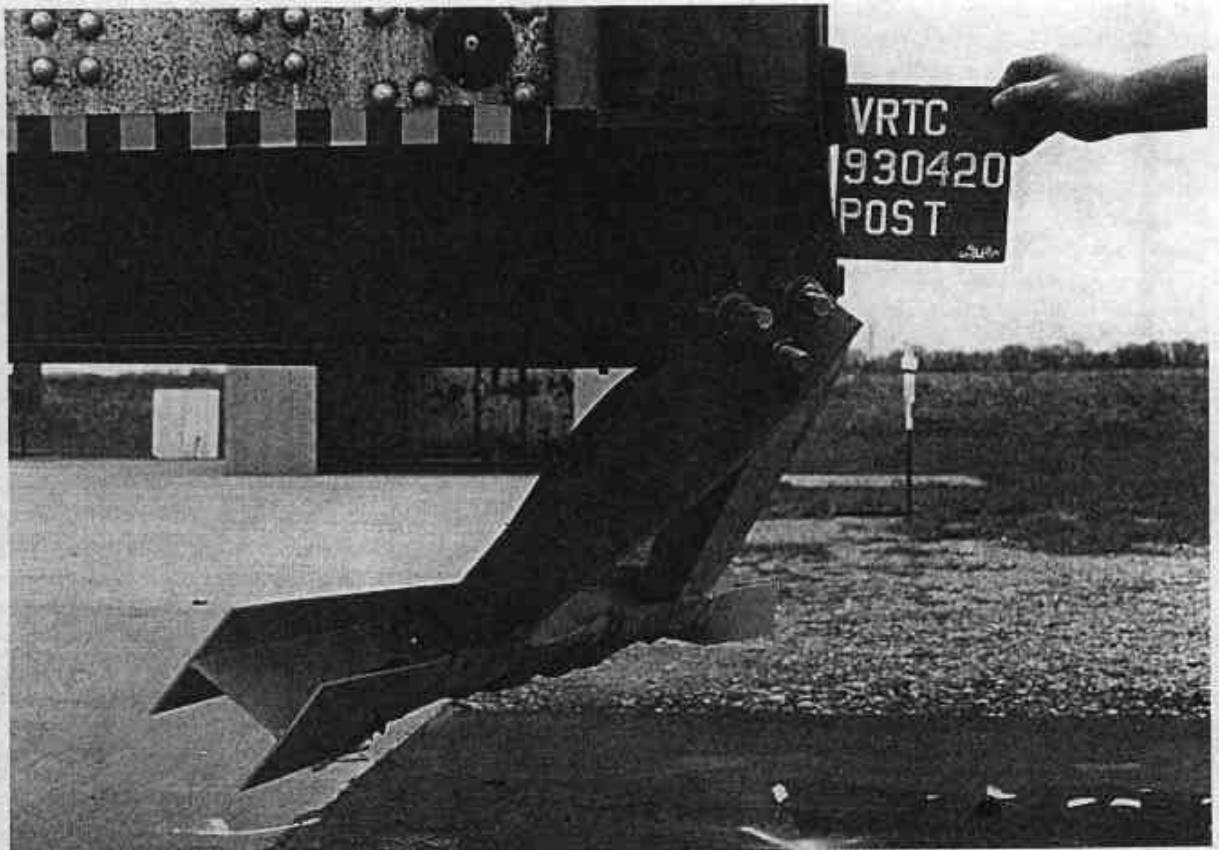
Figure A-42. POST-TEST UNDERRIDE GUARD - VIEW 5
