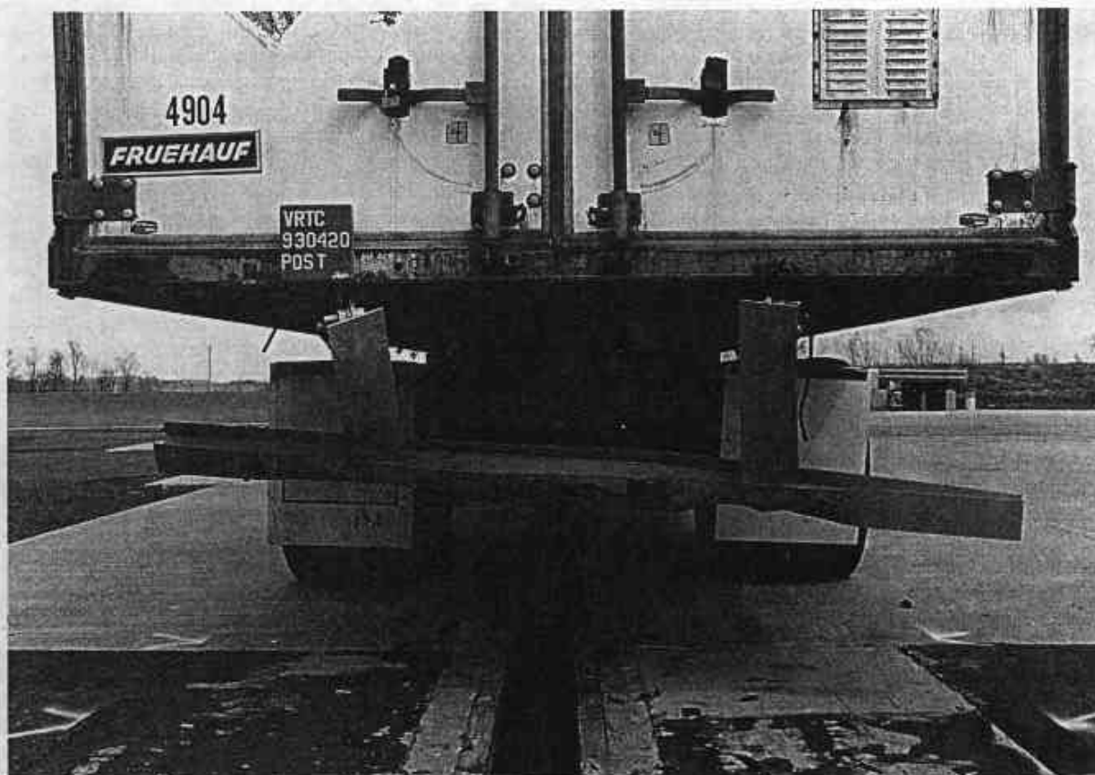
Figure A-38. POST-TEST UNDERRIDE GUARD - VIEW 1
