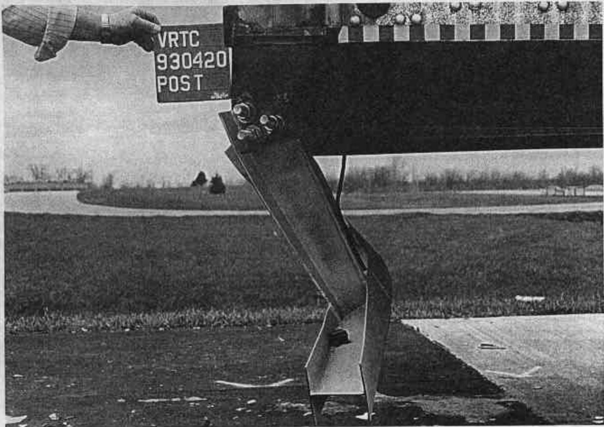
Figure A-39. POST-TEST UNDERRIDE GUARD - VIEW 2
