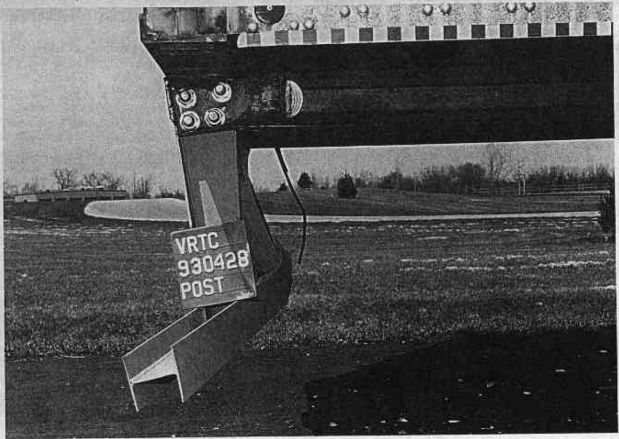
Figure A-37. POST-TEST UNDERRIDE GUARD - VIEW 1
