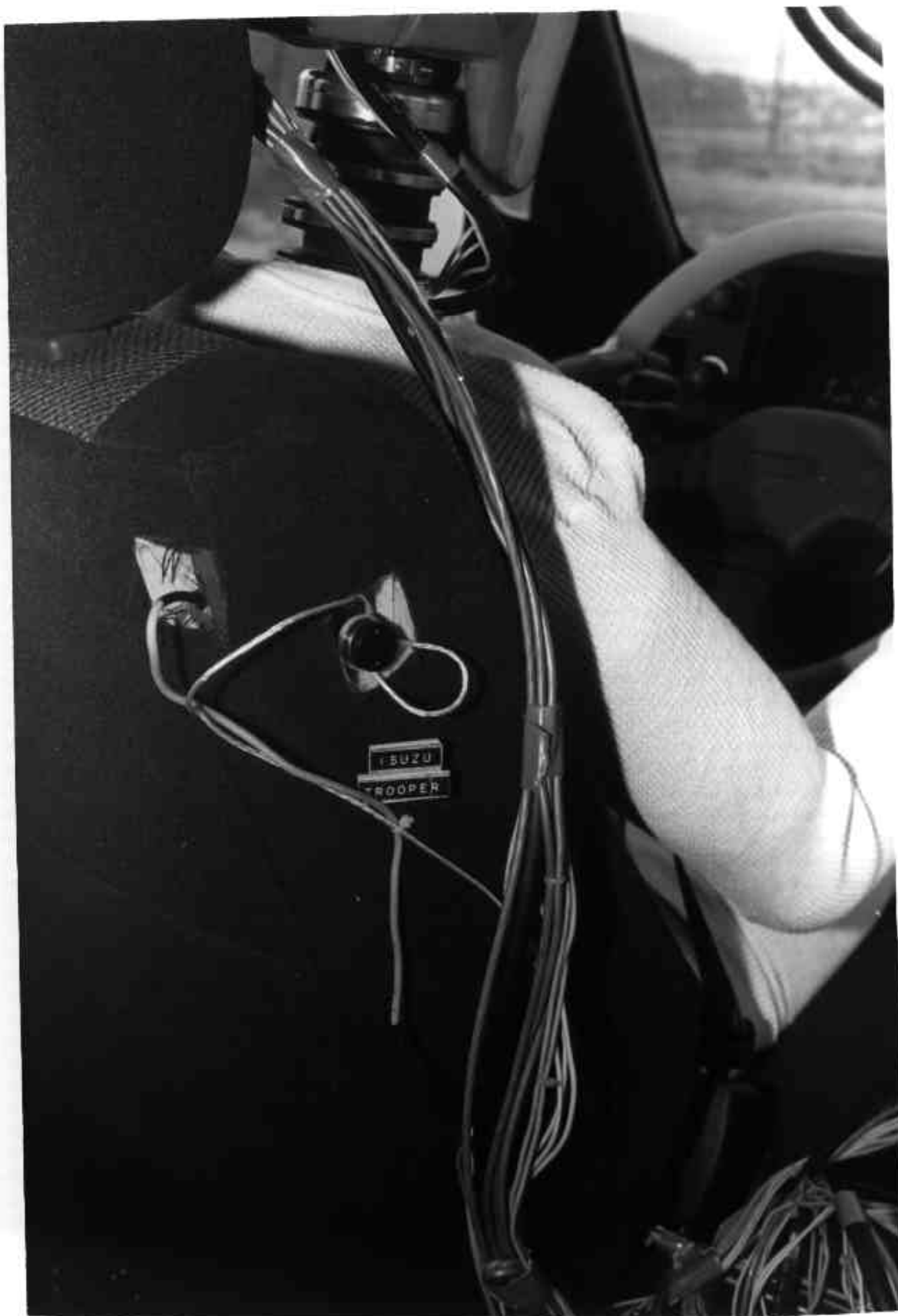
FIGURE 5-16 SEAT FRAME MOUNTED ACCELEROMETER AND MHD SENSOR
