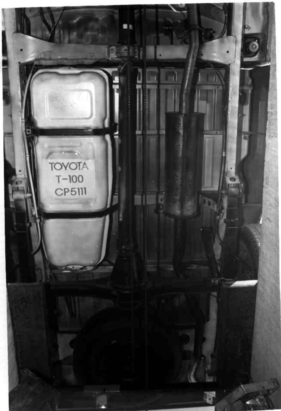
FIGURE 5-10 PRETEST FUEL TANK CLOSEUP VIEW
