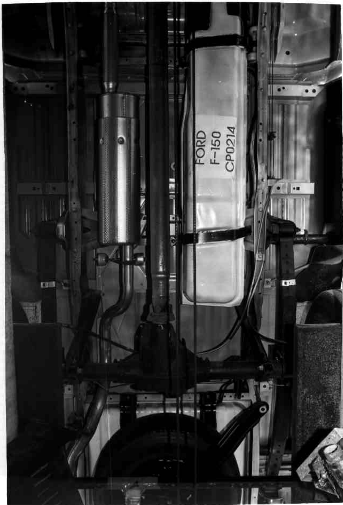
FIGURE 5-10 PRETEST FUEL TANK CLOSEUP VIEW
