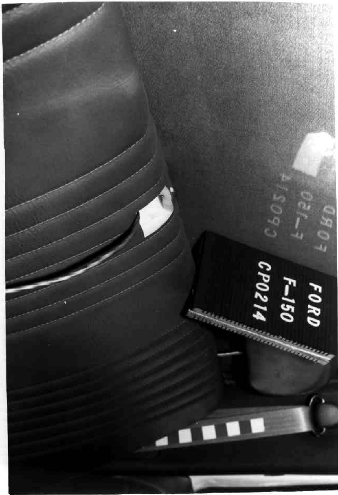
FIGURE 3-17 SEAT FRAME MOUNTED ACCELEROMETER
