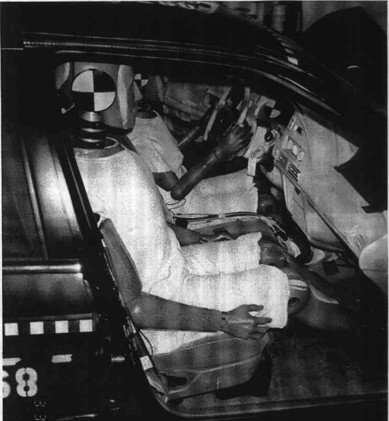
Figure A-34 PRE-TEST PASSENGER AND OCCUPANT COMPARTMENT VIEW
