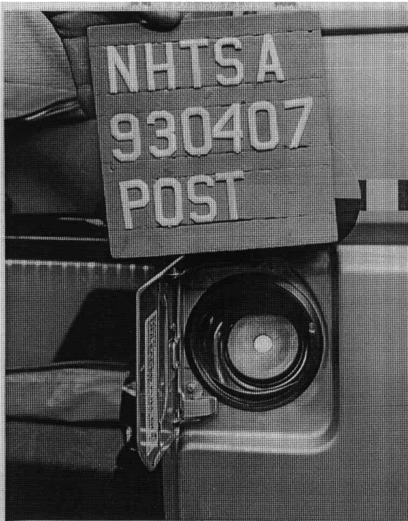
Figure A-18. POST-TEST FUEL FILLER CAP VIEW
