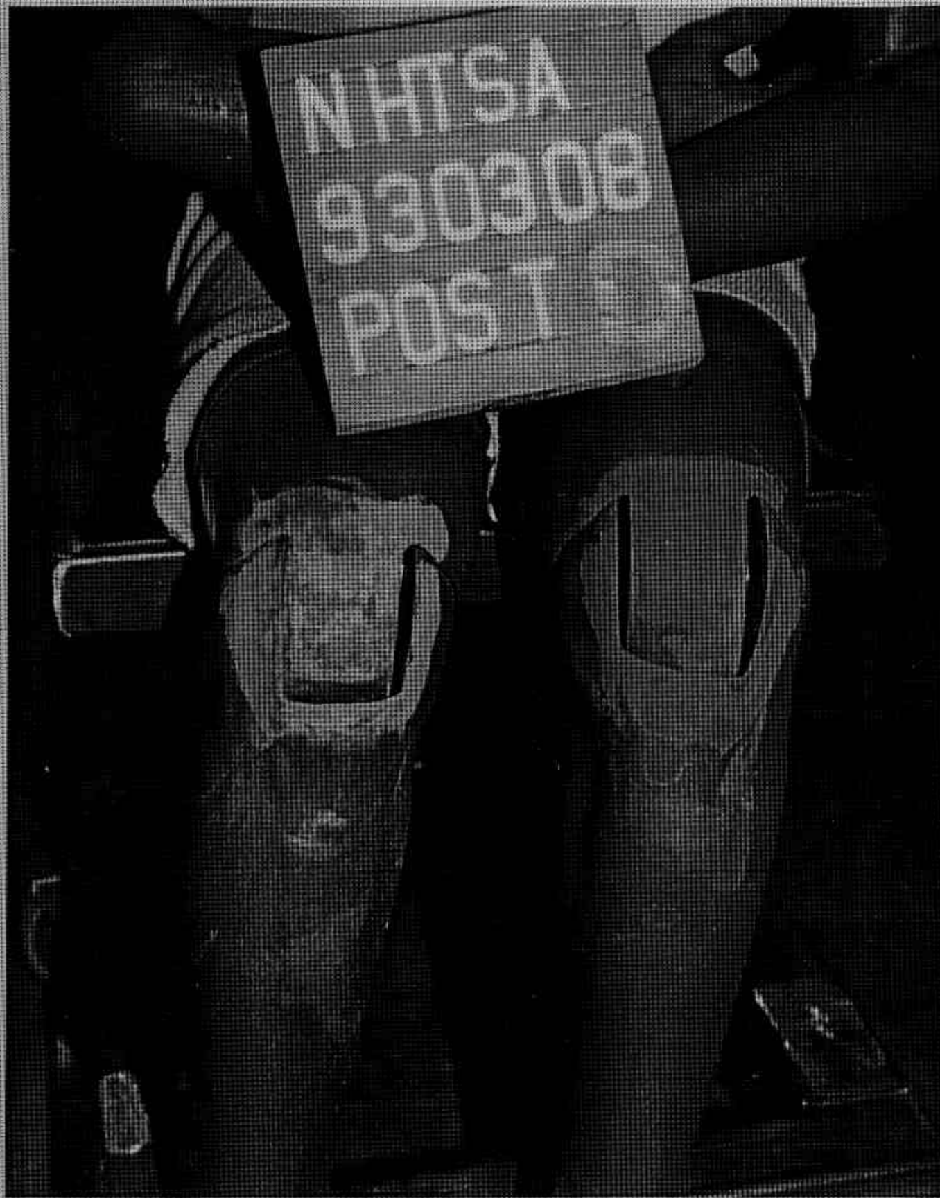
Figure A-39. POST-TEST DRIVER DUMMY KNEE CONTACT - VIEW 1
