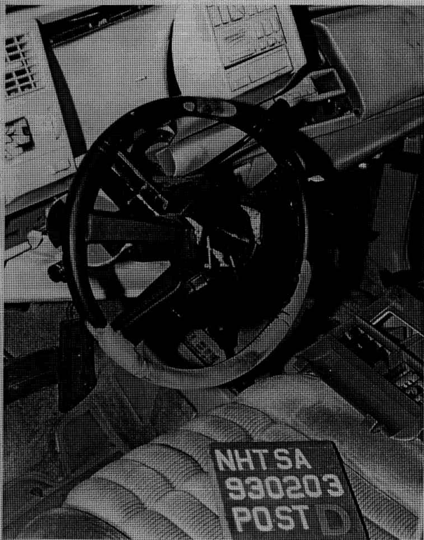
Figure A-41. POST-TEST DRIVER DUMMY HEAD & CHEST CONTACT VIEW
