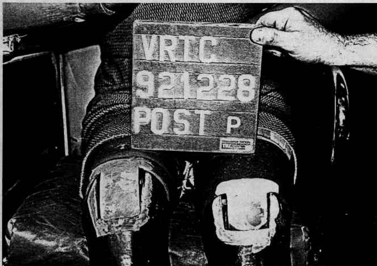
Figure A-40. POST-TEST PASSENGER DUMMY KNEE CONTACT - VIEW 1
