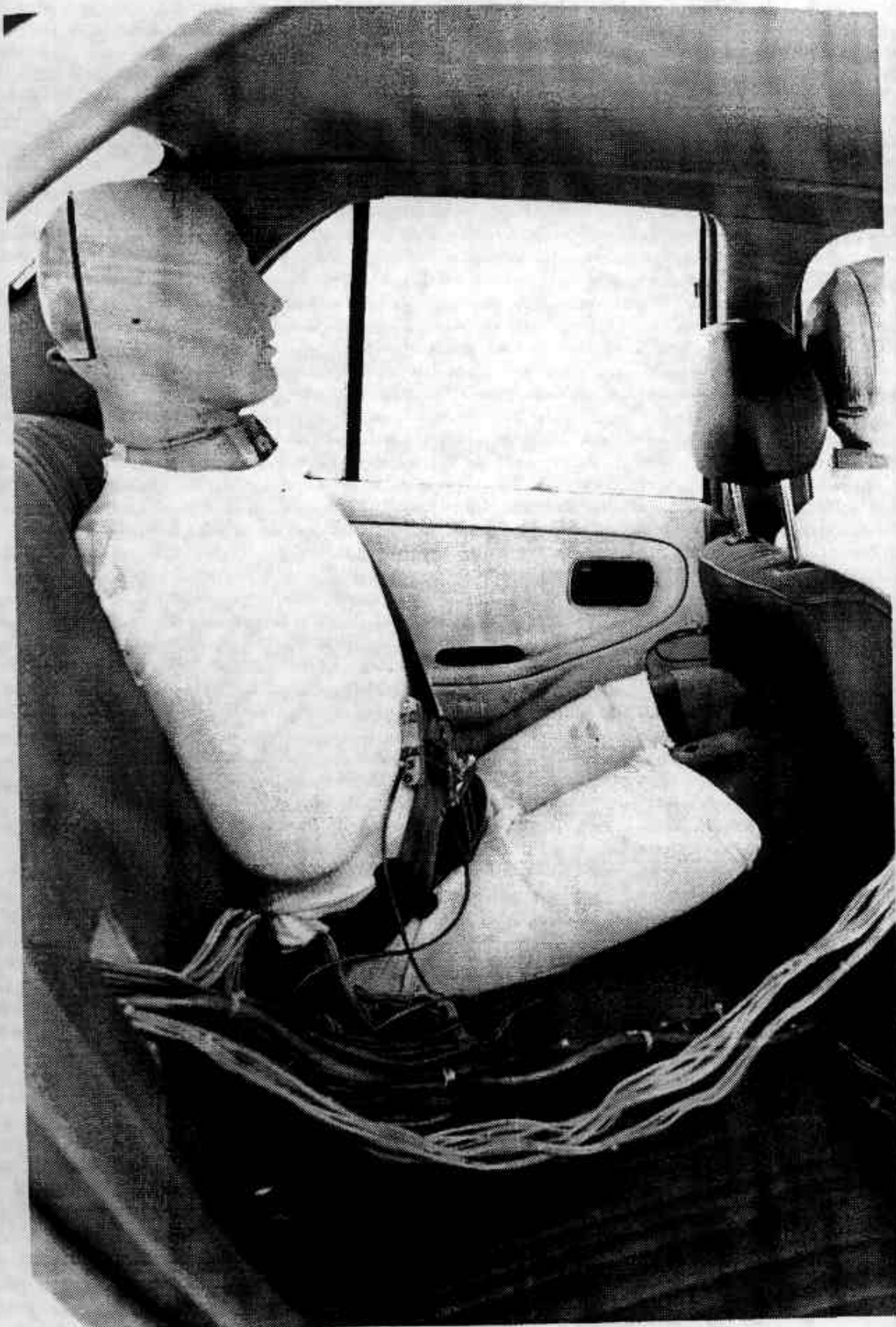
FIGURE 5-21 PRETEST OCCUPANT COMPARTMENT RIGHT SIDE VIEW SHOWING PASSENGER SID
