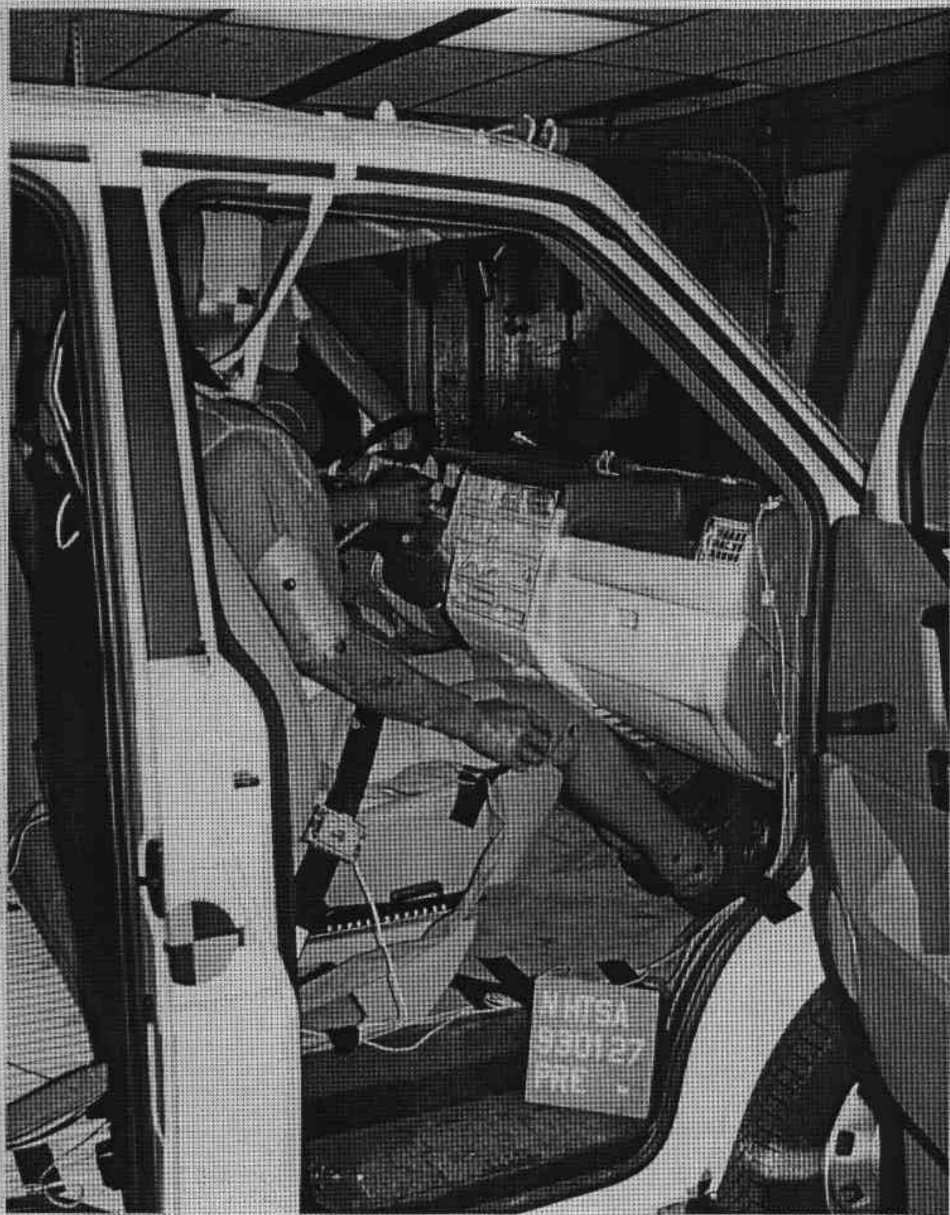
Figure A-35. PRE-TEST PASSENGER DUMMY & VEHICLE INTERIOR - VIEW I
