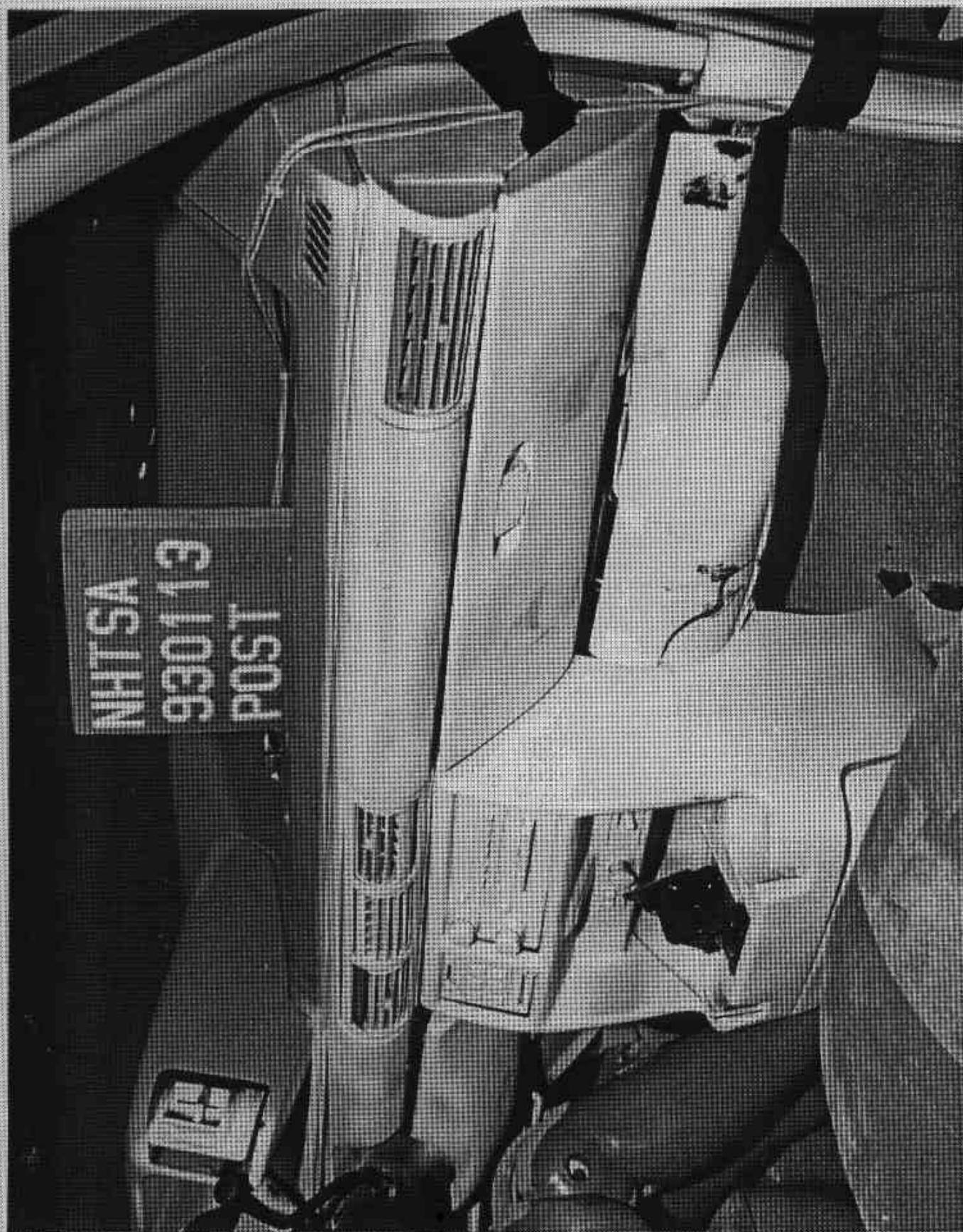
Figure A-45. POST-TEST PASSENGER DUMMY KNEE CONTACT - VIEW 2 A-46 930113
