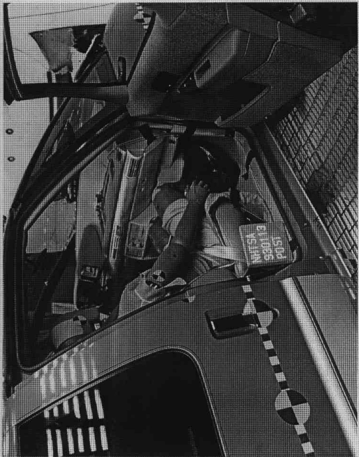
Figure A-36. POST-TEST PASSENGER DUMMY & VEHICLE INTERIOR - VIEW 1 A-37 930113
