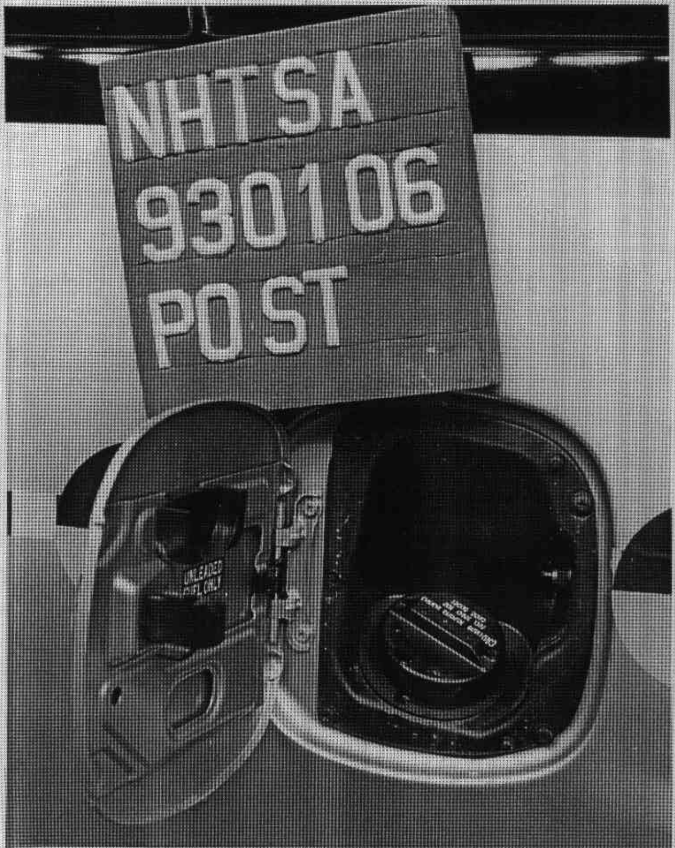
Figure A-18. POST-TEST FUEL FILLER CAP VIEW
