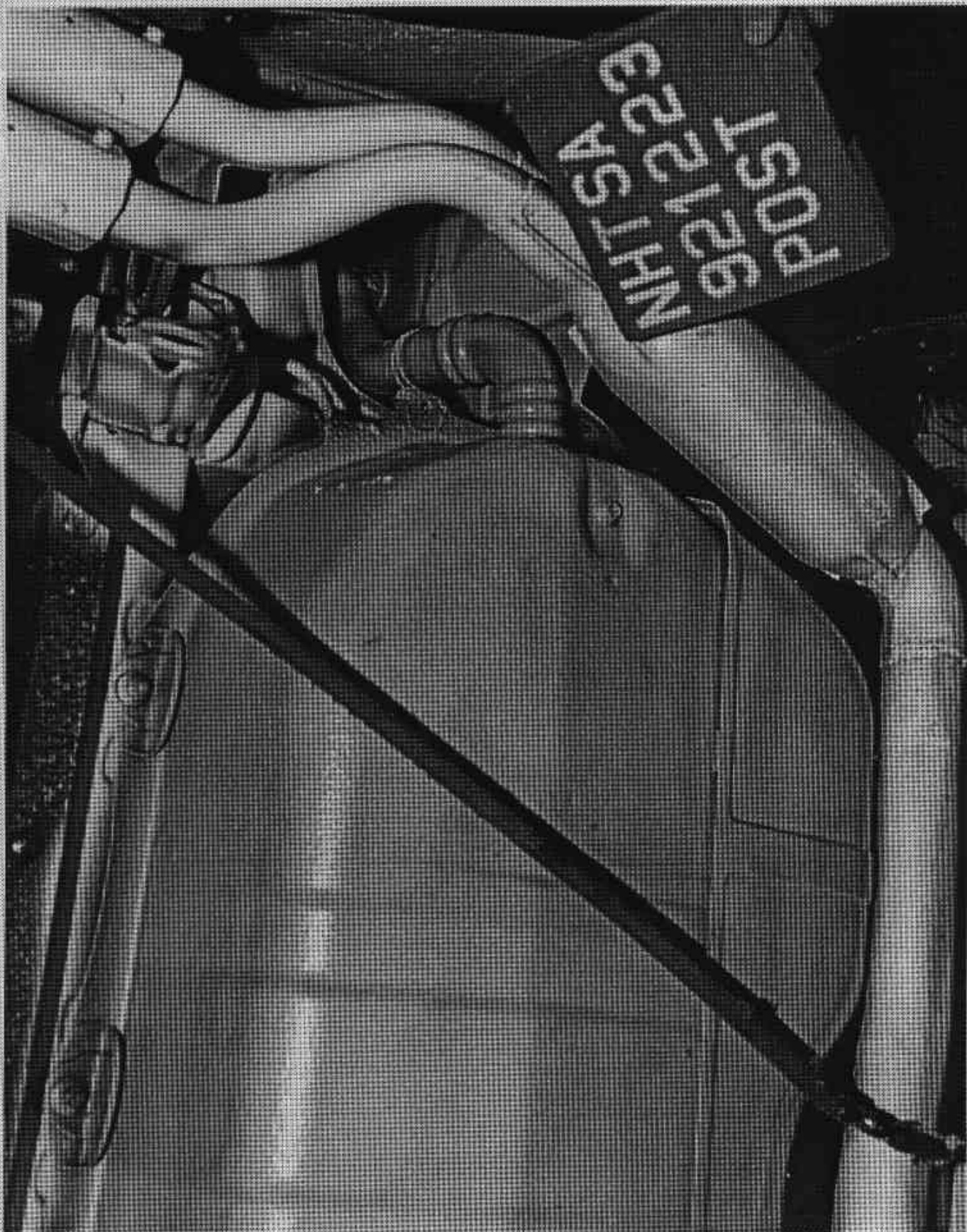
FIGURE A-20. POST-TEST FUEL FILLER NECK VIEW
