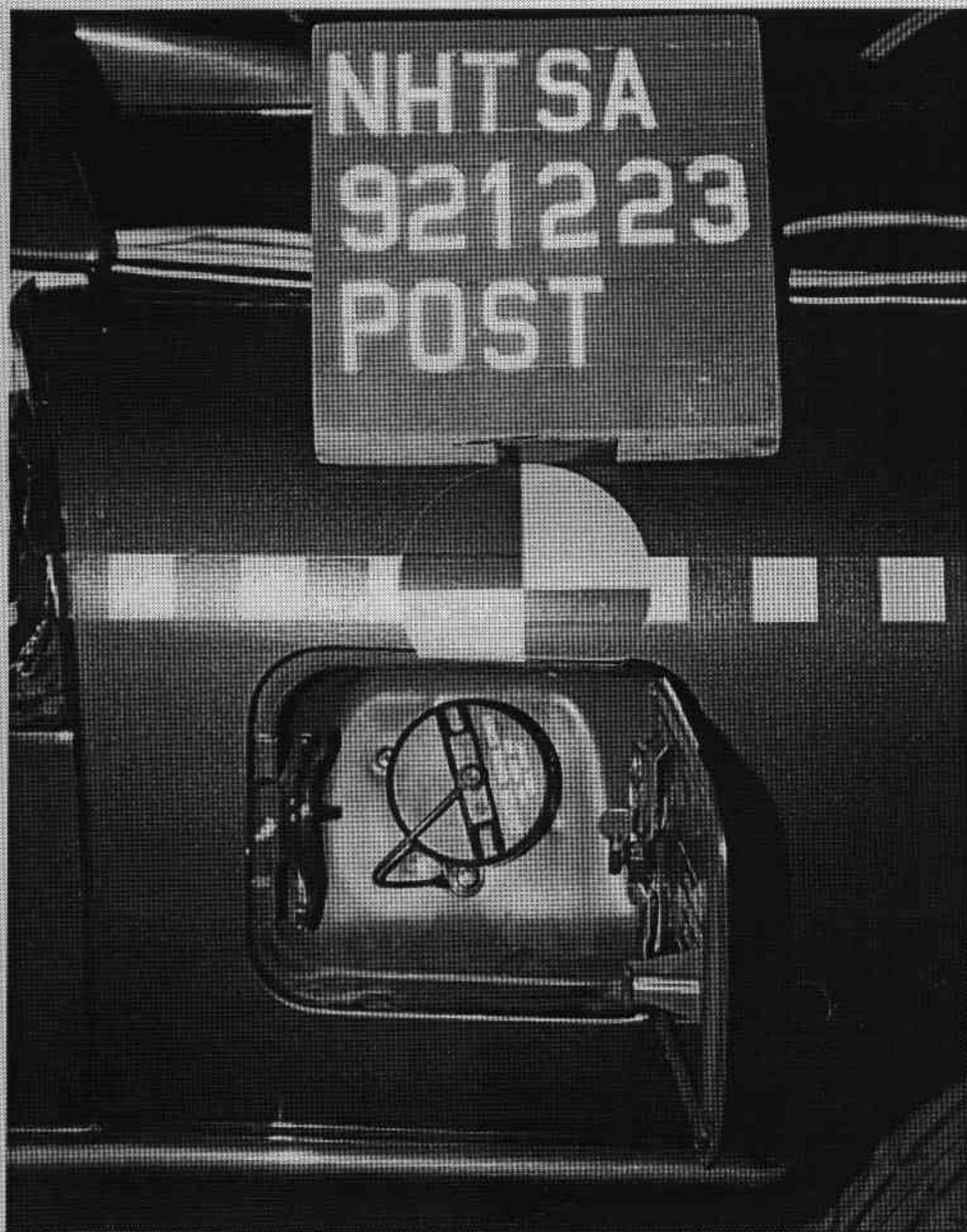
FIGURE A-18. POST-TEST FUEL FILLER CAP VIEW
