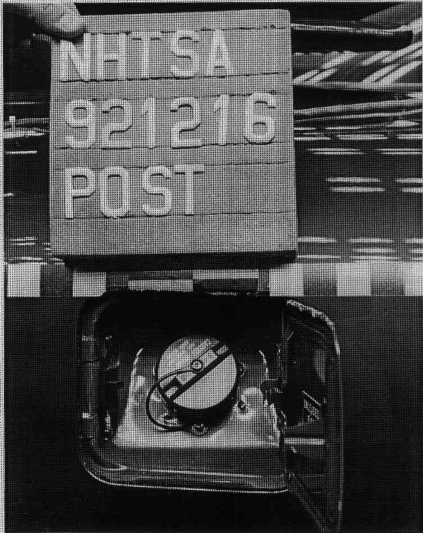
FIGURE A-18. POST-TEST FUEL FILLER CAP VIEW A-19
