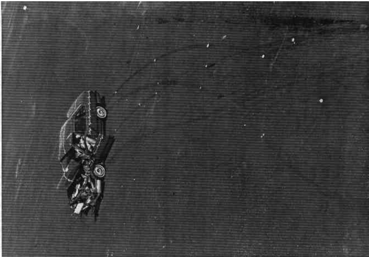
Figure A-45. POST-TEST VEHICLE SKID MARKS - VIEW 1
