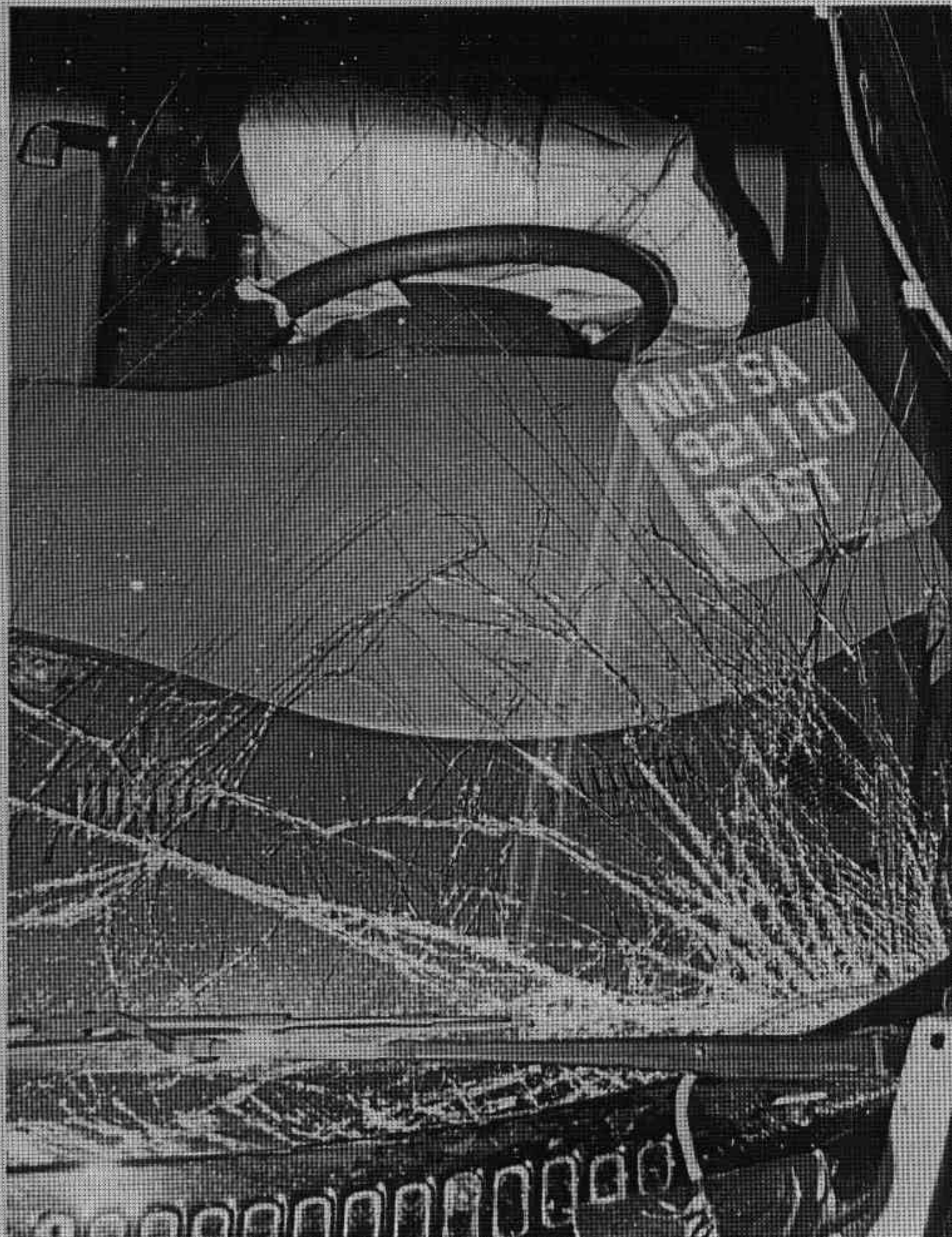
FIGURE A-49. POST-TEST STEERING COLUMN POSITION - VIEW 2
