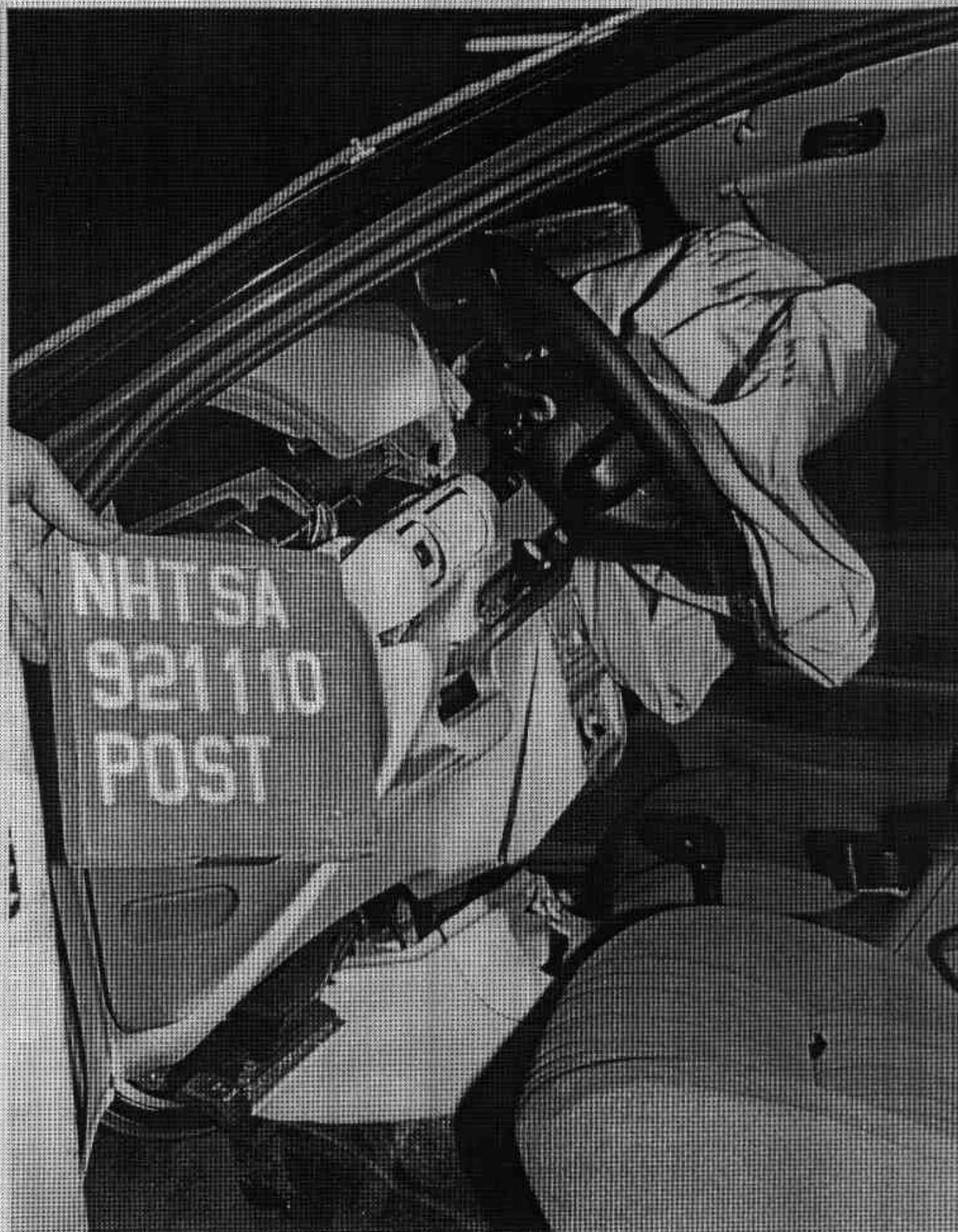
FIGURE A-50. POST-TEST STEERING COLUMN POSITION - VIEW 3
