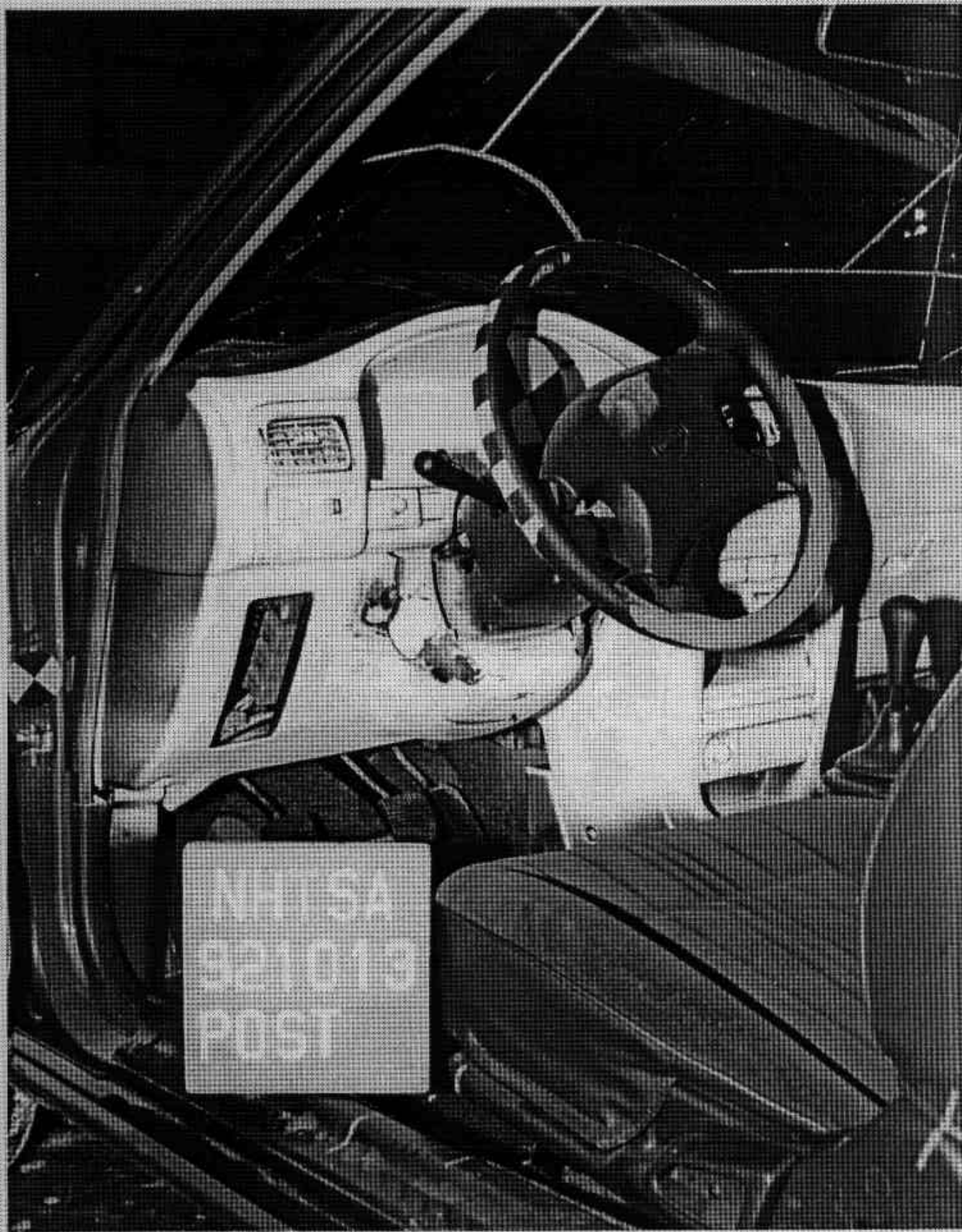
FIGURE A-40, POST-TEST DRIVER DUMMY HEAD & KNEE CONTACT VIEW
